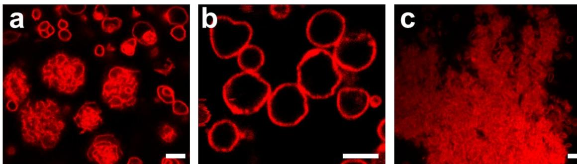
**Figure S4.** LSM images of structures formed by polymers (a) ABC-biotin (PEO<sub>45</sub>-*b*-PCL<sub>103</sub>-*b*-PMOXA<sub>4</sub>-biotin), (b) ABC (PEO<sub>45</sub>-*b*-PCL<sub>110</sub>-*b*-PMOXA<sub>4</sub>), (c) PEO<sub>45</sub>-*b*-PCL<sub>135</sub>-*b*-PMOXA<sub>20</sub>. ABC-biotin forms a mixture of polymersomes and cloud-like aggregates indicating that the packing geometry of ABC-biotin molecules is somewhat intermediate between cylinder
