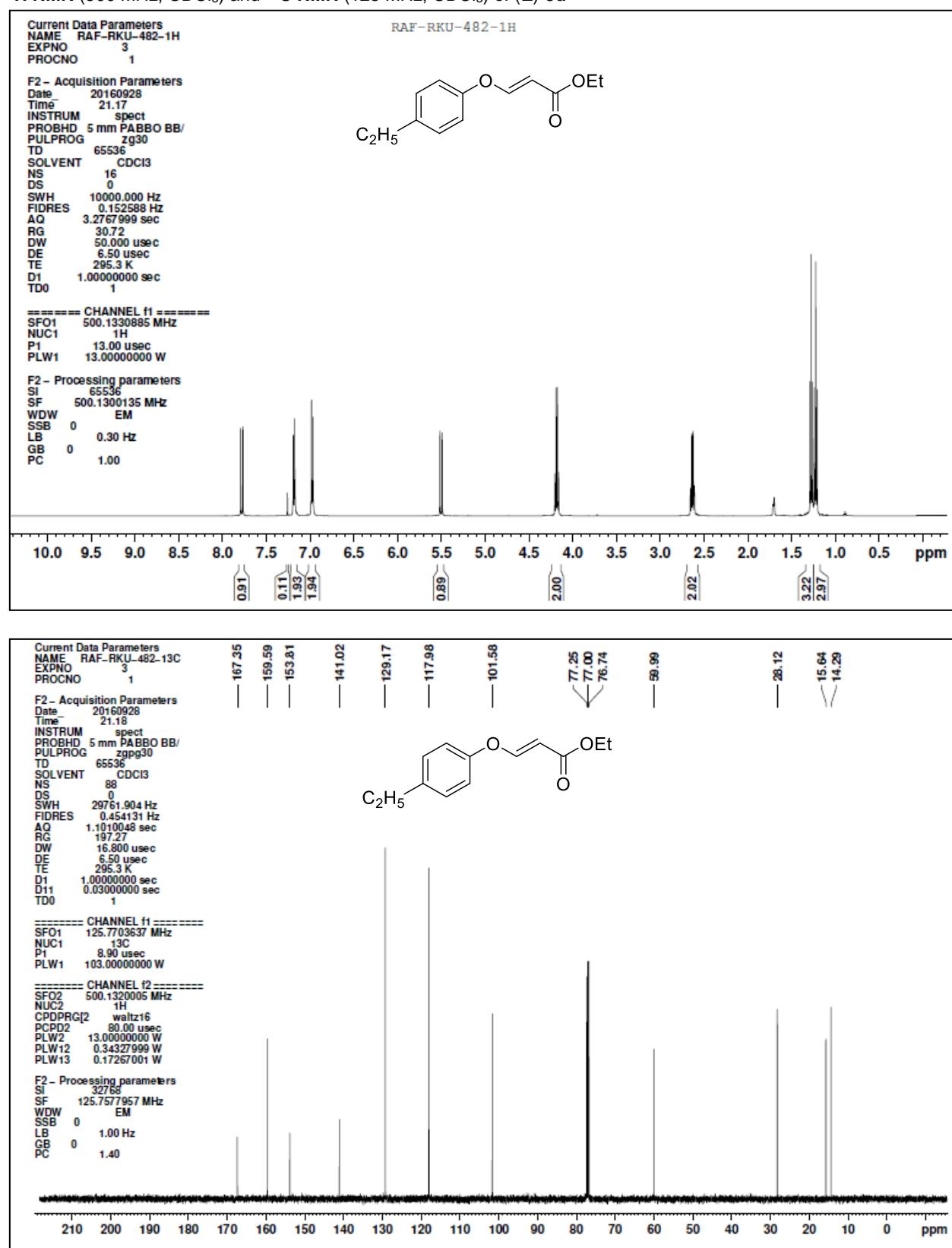
**<sup>1</sup>H NMR (400 MHz, CDCl<sub>3</sub>) and <sup>13</sup>C NMR (100 MHz, CDCl<sub>3</sub>) of (*E*)-3e**
