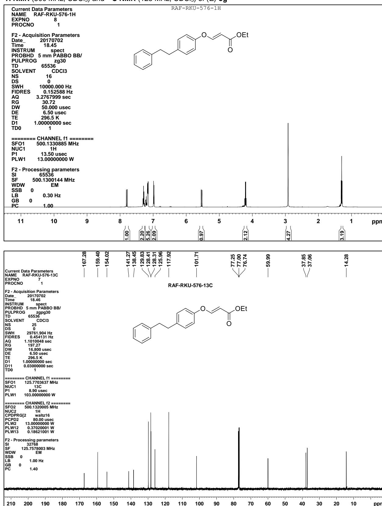
**<sup>1</sup>H NMR (500 MHz, CDCl<sub>3</sub>) and <sup>13</sup>C NMR (125 MHz, CDCl<sub>3</sub>) of (*E*)-3h**
