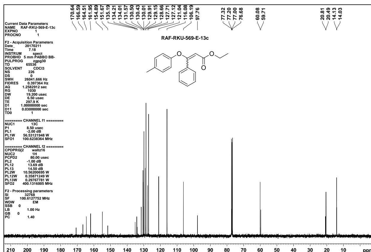
**<sup>1</sup>H NMR (500 MHz, CDCl<sub>3</sub>) and <sup>13</sup>C NMR (125 MHz, CDCl<sub>3</sub>) of 24**
