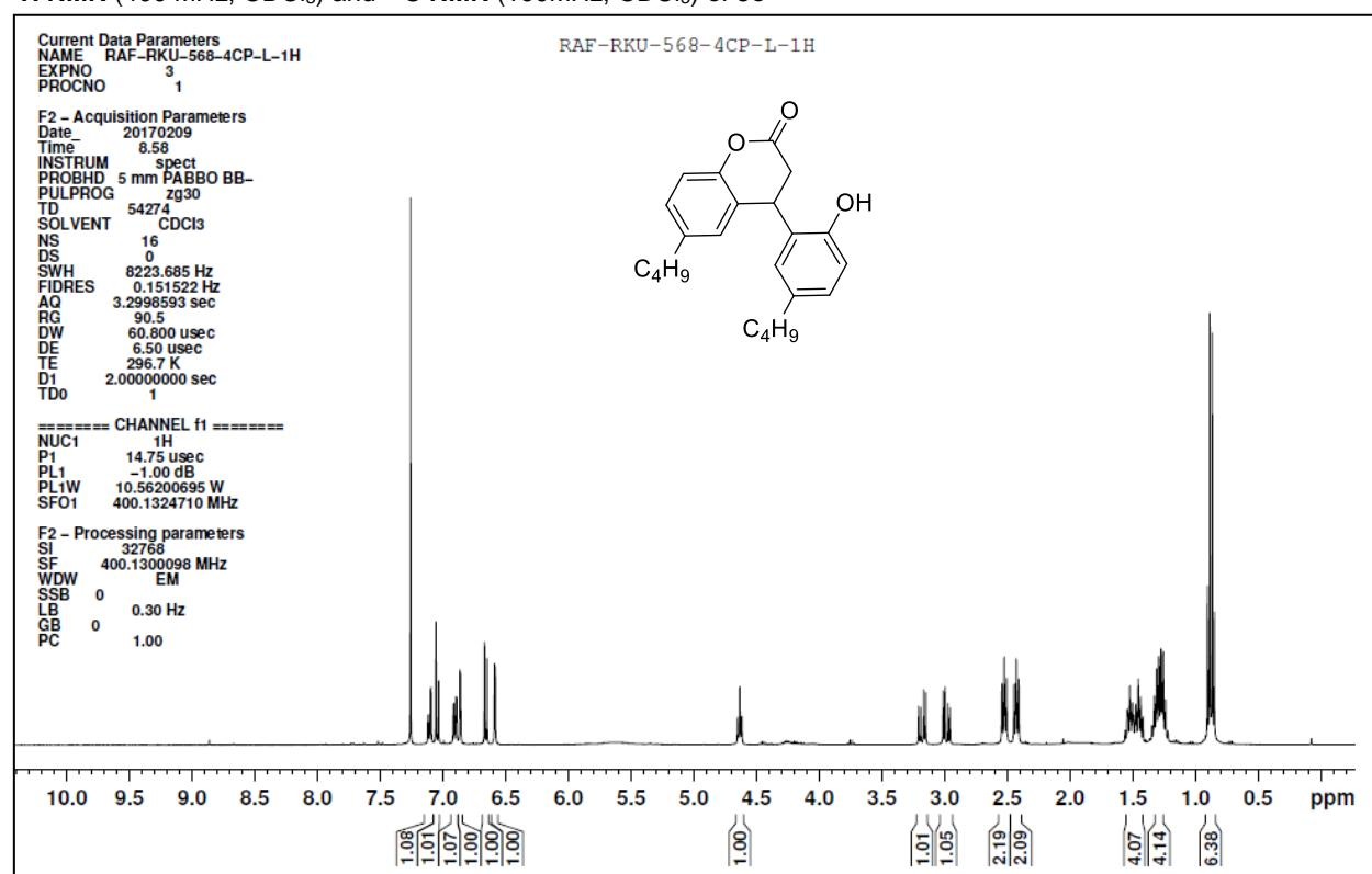
**<sup>1</sup>H NMR** (400 MHz, CDCl<sub>3</sub>) and **<sup>13</sup>C NMR** (125 MHz, CDCl<sub>3</sub>) of **5f**
