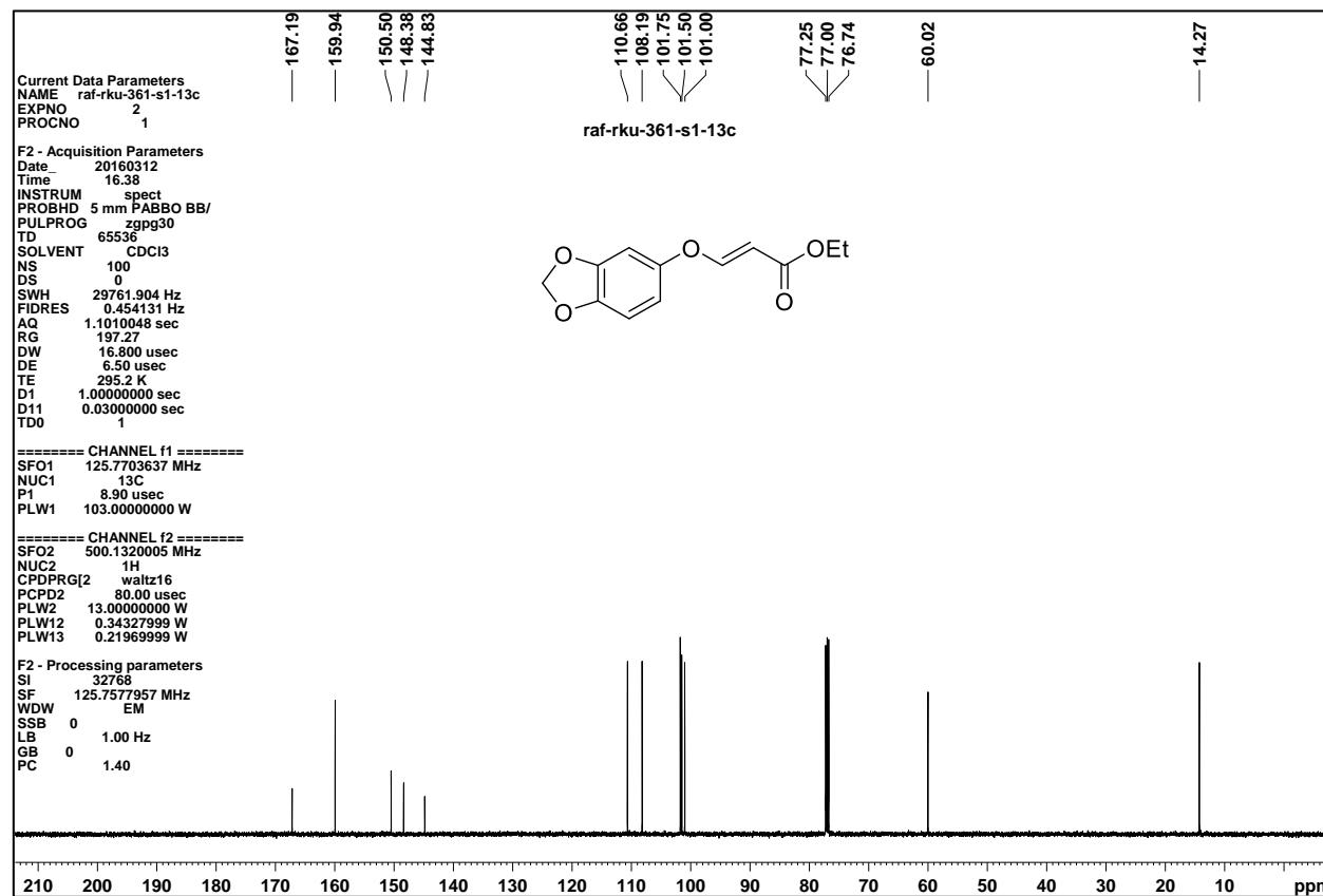
**<sup>1</sup>H NMR (400 MHz, CDCl<sub>3</sub>) and <sup>13</sup>C NMR (100 MHz, CDCl<sub>3</sub>) of (*E*)-3q**
