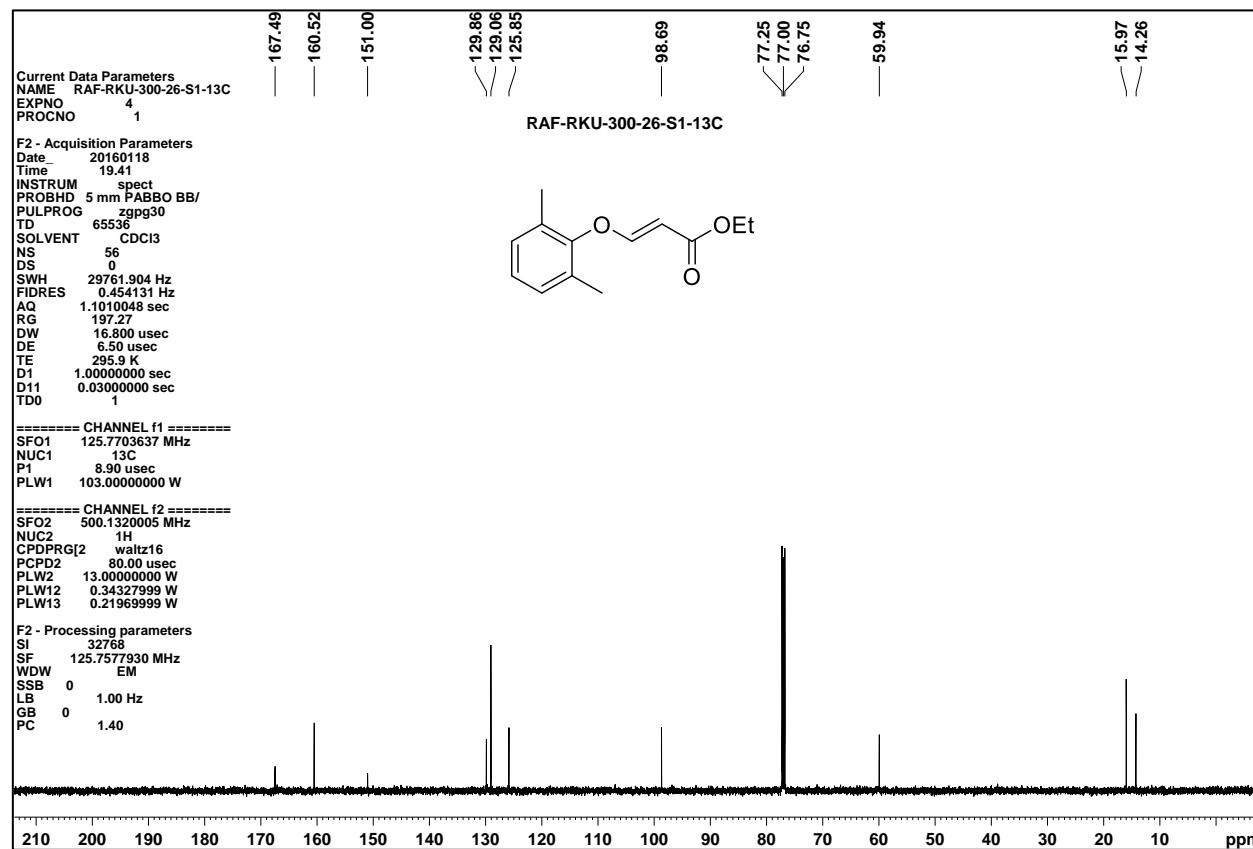
**<sup>1</sup>H NMR (400 MHz, CDCl<sub>3</sub>) and <sup>13</sup>C NMR (100 MHz, CDCl<sub>3</sub>) of (*E*)-3y**
