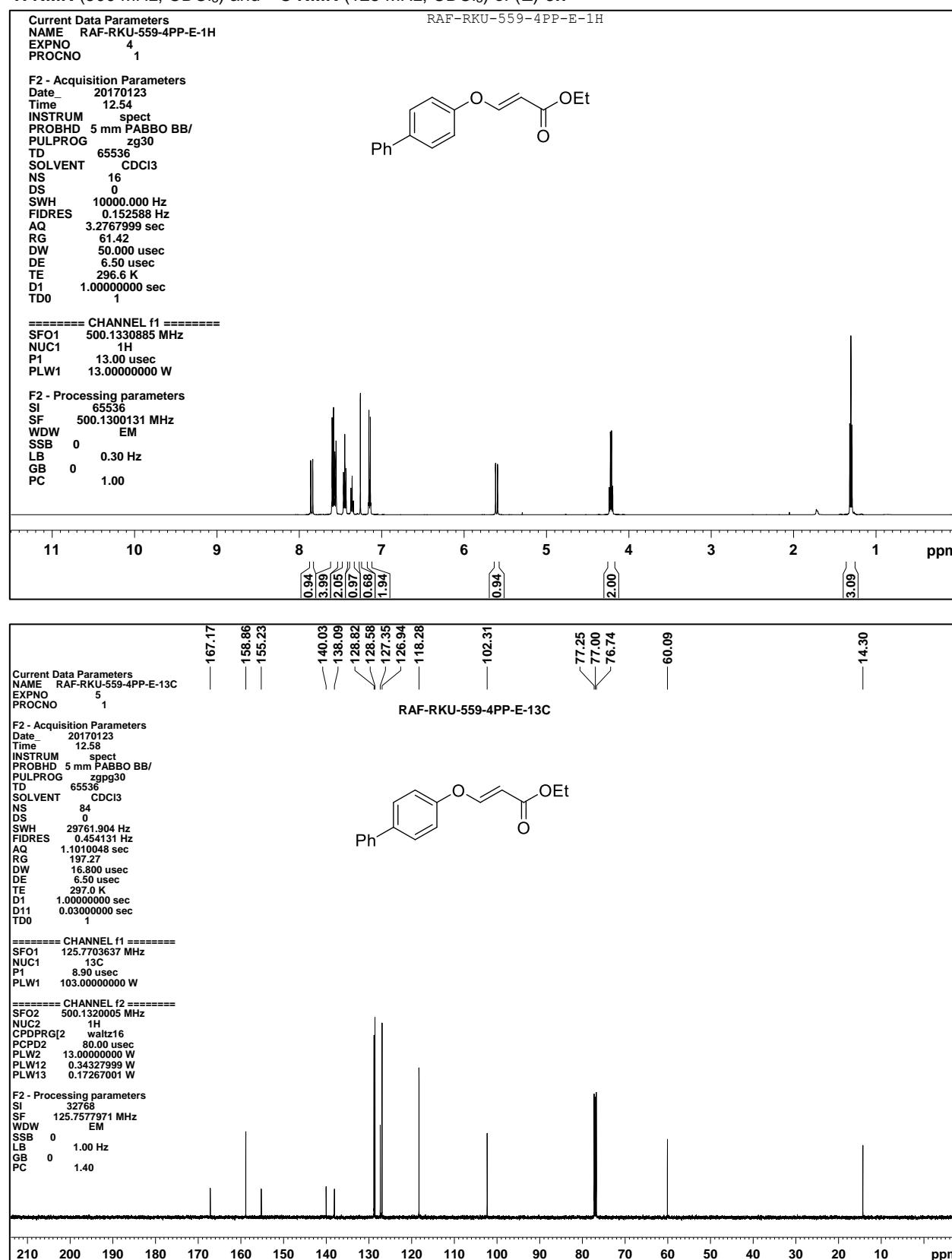
**<sup>1</sup>H NMR (400 MHz, CDCl<sub>3</sub>) and <sup>13</sup>C NMR (100 MHz, CDCl<sub>3</sub>) of (*E*)-3i**
