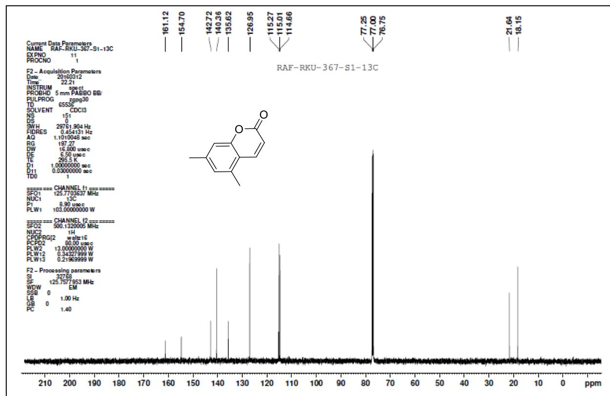
**<sup>1</sup>H NMR (400 MHz, CDCl<sub>3</sub>) and <sup>13</sup>C NMR (100 MHz, CDCl<sub>3</sub>) of 5p**
