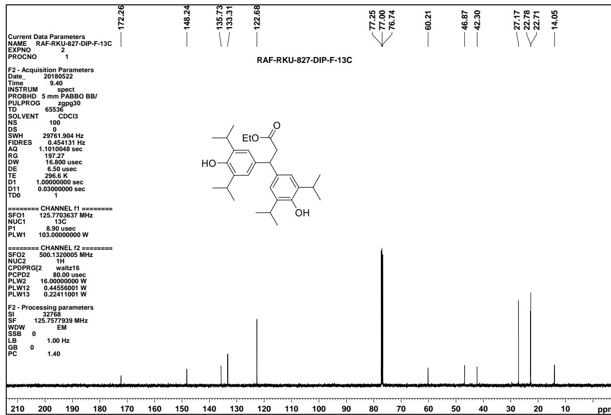
**<sup>1</sup>H NMR (400 MHz, CDCl<sub>3</sub>) and <sup>13</sup>C NMR (100 MHz, CDCl<sub>3</sub>) of 5z**
