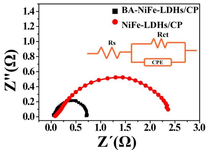
**Figure S9** Nyquist plots of BA-NiFe-LDHs/CP and NiFe-LDHs/CP. Inset: an equivalent circuit used for fitting data.
