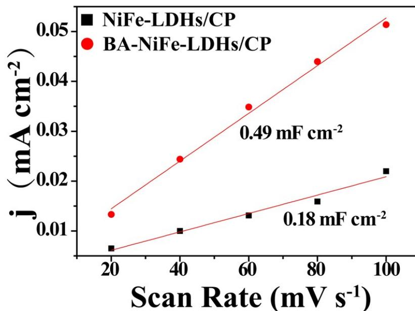
**Figure S13** The capacitive currents at 0.075 V vs. SCE as a function of scan rate for electrodes. The determined double-layer capacitance of the system is taken as the average of the absolute value of the slope for the linear fits to the data.
