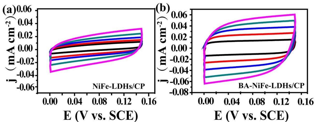
Figure S12 CVs of (a) NiFe-LDHs/CP and (b) BA-NiFe-LDHs/CP in the non-faradaic capacitance current range at scan rates of 20, 40, 60, 80, and 100  $\text{mV s}^{-1}$
