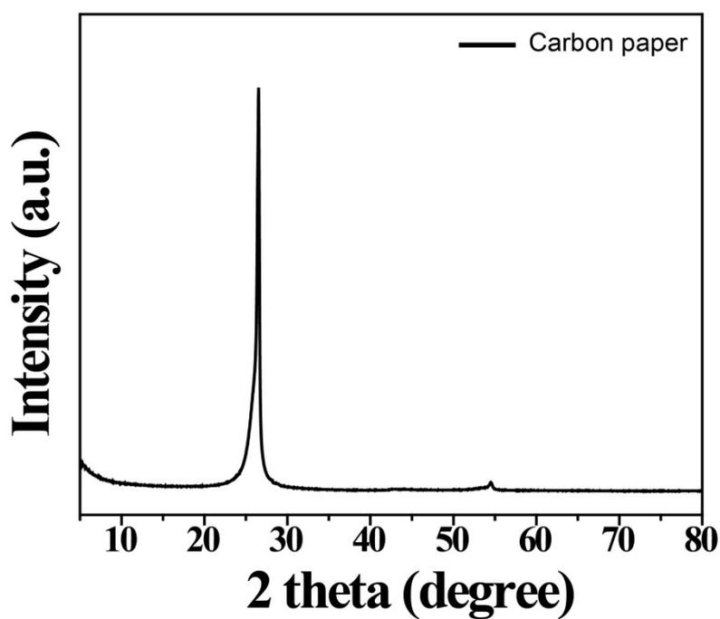
Figure S1 XRD patterns of carbon paper.
