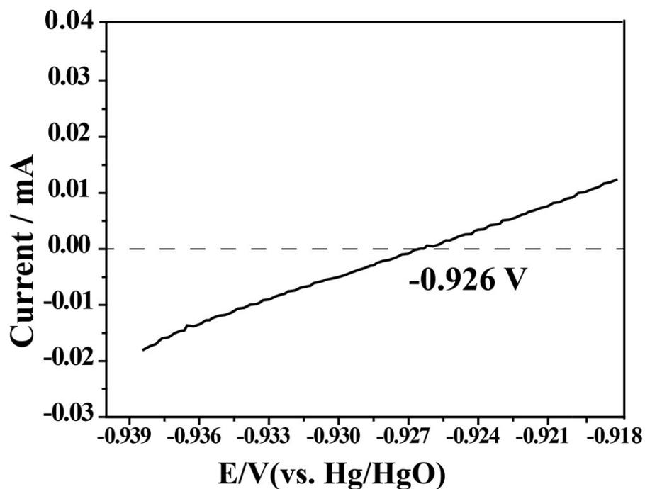
**Figure S6** The LSV curves of hydrogen electrode reactions on Pt wire.
