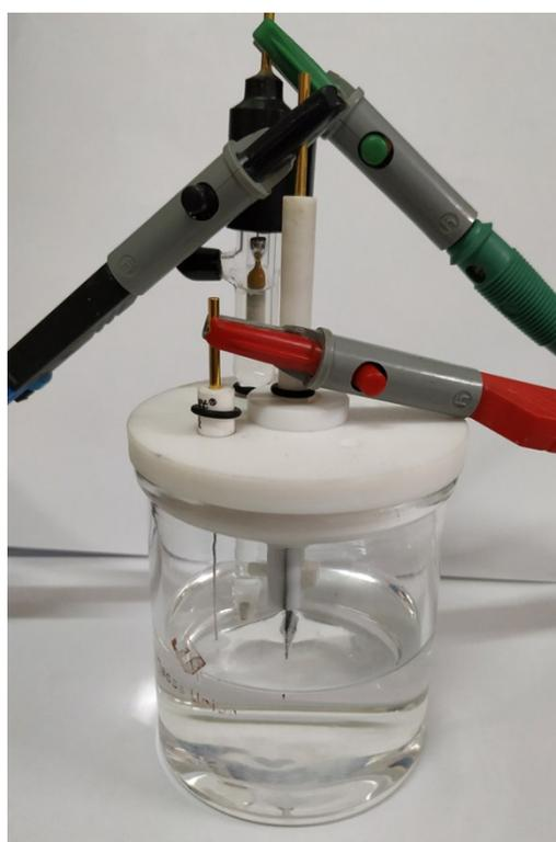
**Figure S5** The digital image of electrolytic cell with electrode.
