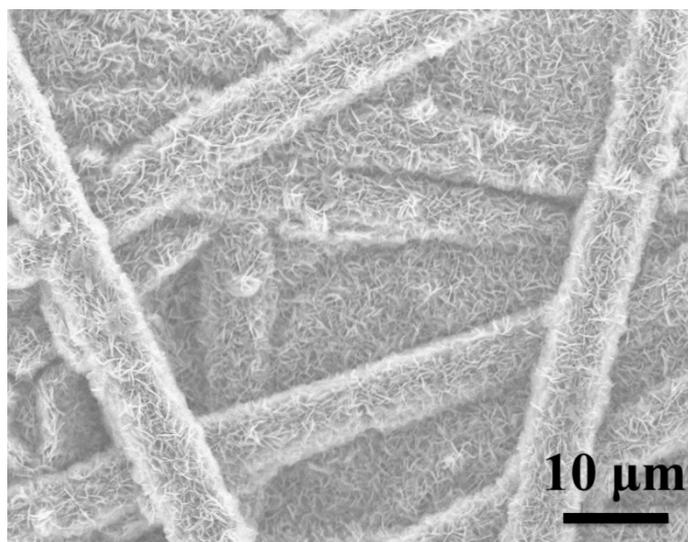
**Figure S10** SEM of BA-NiFe-LDHs/CP after stability test in 1.0 M KOH.
