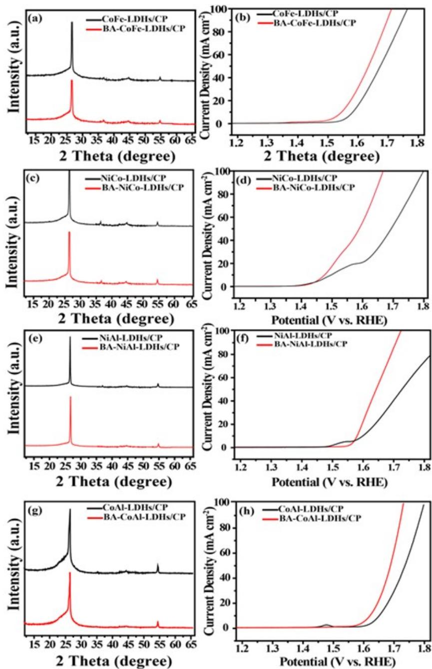
**Figure S8** the XRD patterns and the polarization curves for the OER in 1.0 M KOH solution (scan rate  $5 \text{ mV s}^{-1}$ ) of CoFe-LDHs/CP and BA-CoFe-LDHs/CP (a), (b); NiCo-LDHs/CP and BA-NiCo-LDHs/CP (c), (d); NiAl-LDHs/CP and BA-NiAl-LDHs/CP (e), (f) ; CoAl-LDHs/CP and BA-CoAl-LDHs/CP (g), (h) ,respectively.
