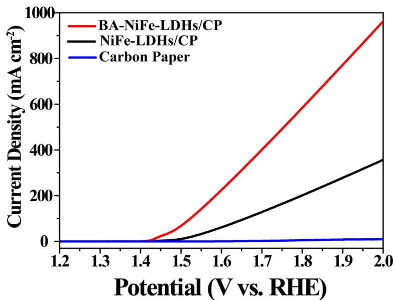
**Figure S7** The polarization curves of CP, NiFe-LDHs/CP and BA-NiFe-LDHs/CP for the OER in 1.0 M KOH solution (scan rate 5 mV s<sup>-1</sup>)
