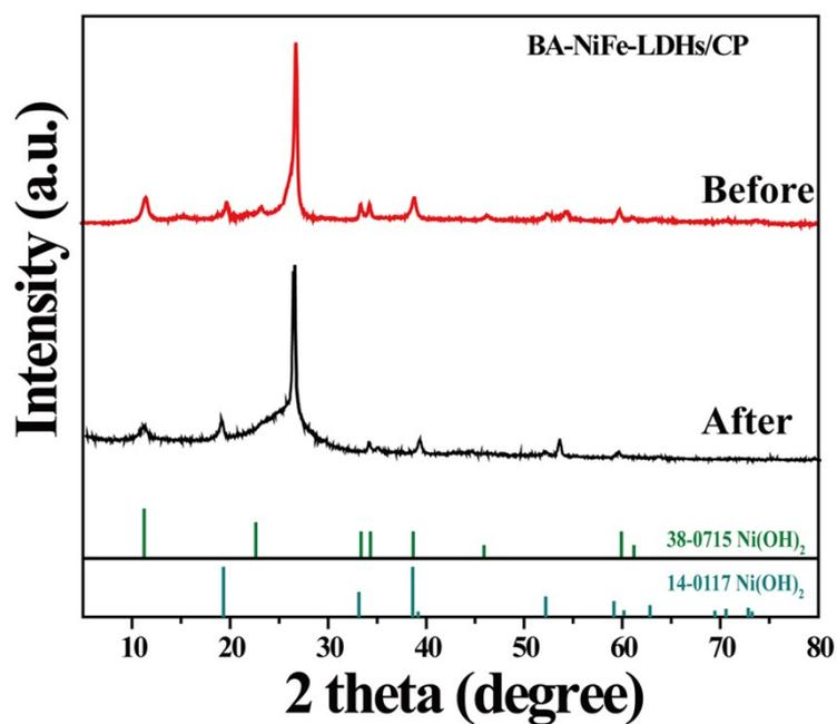
Figure S11 The XRD of the BA-NiFe-LDHs /CPbefore and after durability tests.
