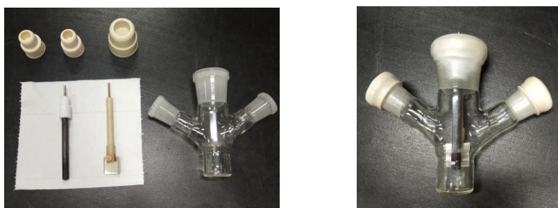
Figure S1. The experimental setup for electrolysis.
