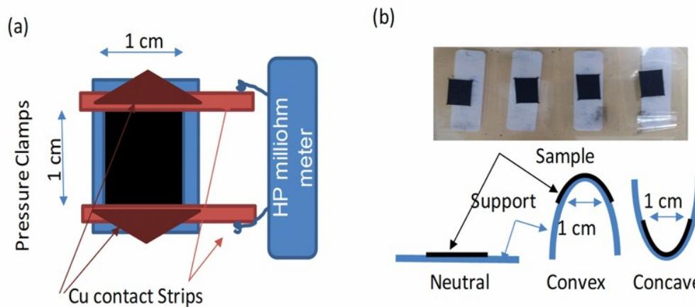
**Fig. S8** The schematic diagram of equipment for testing mechanical strength (flexibility) of low temperature carbon paste film. (b) the preparation of the sample and the diagram of bending state and bending angle.<sup>2</sup>
