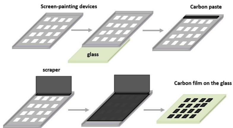
**Fig. S2** The manufacturing process of screen-printing carbon.
