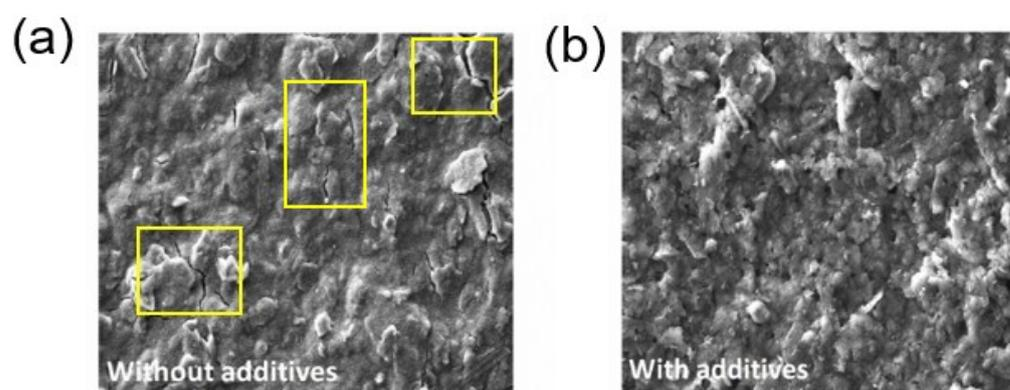
**Fig. S6** The surface SEM characterization of low temperature carbon film without the treatment (a) and with the treatment of mixed functional additives (b).
