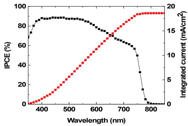
**Fig. S4** The IPCE and integrated current density of the typical solar cell device.
