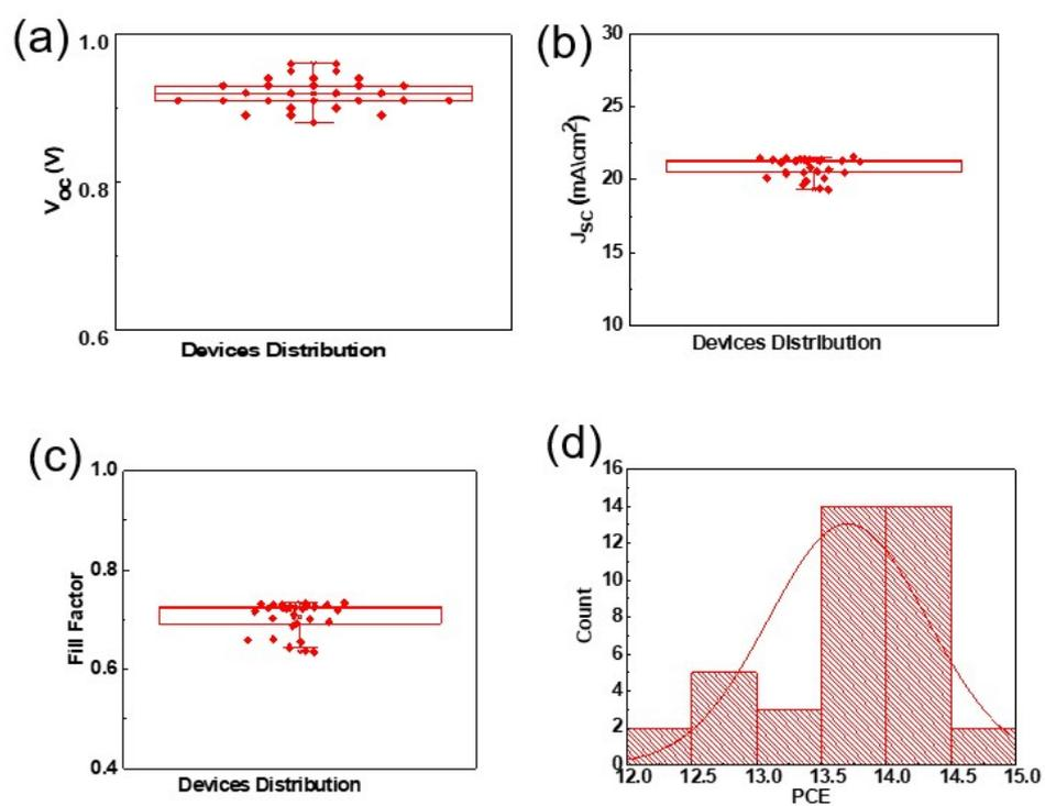
**Fig. S5** The box diagram of  $V_{OC}$  (a),  $J_{SC}$  (b), FF (c) about the parameters of battery performance, (d) the histogram bar graph and normal distribution of PCE about 40 pieces of perovskite solar cells.
