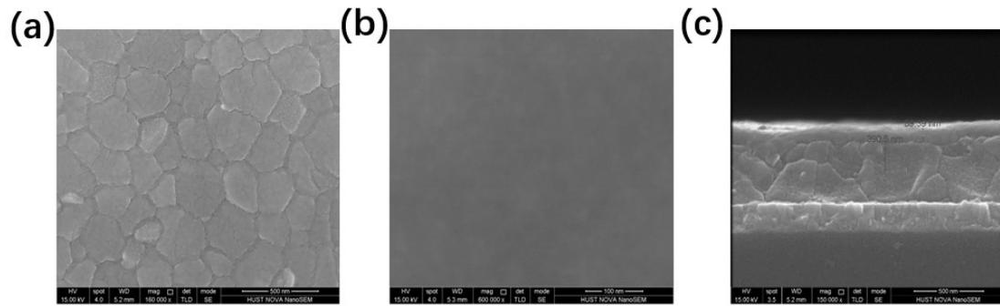
**Fig. S7** (a) The surface SEM characterization of perovskite. (b)The surface SEM characterization of PEDOT: PSS. (c) The cross section SEM image of the ITO/perovskite/PEDOT: PSS on glass.
