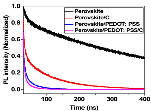
**Fig. S3** The TRPL decays of perovskite film, perovskite/C, perovskite/PEDOT: PSS, and perovskite/PEDOT: PSS/C.
