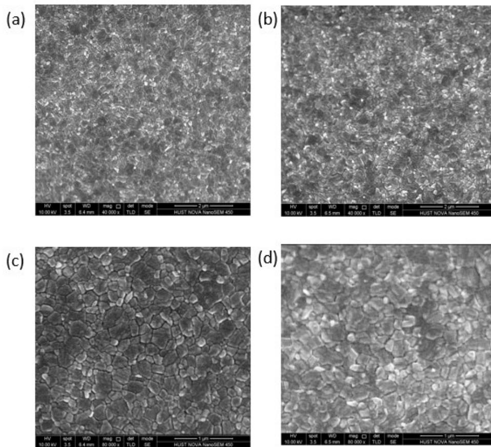
**Fig. S1** (a-d) The surface SEM image of the perovskite film before and after treatment with component solvents.
