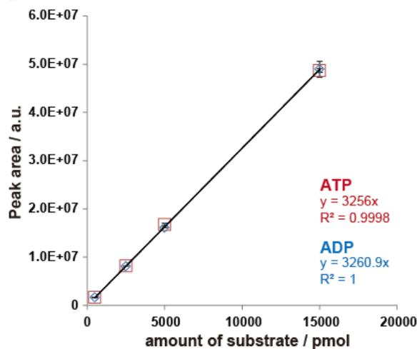
**Fig. S7** (A) Quantitation of the peak area for given concentration and injection volume (100, 500, 1000, and 3000  $\mu\text{M}$ , 5  $\mu\text{L}$ ) of ATP and ADP measured by HPLC analysis. The values were used for calculating standard curves for the quantitation of the creatine phosphokinase reaction. (B) The quantitative titration curves for conversion from the peak area to the amount of substrate, ATP (pink squares) and ADP (blue diamonds).
