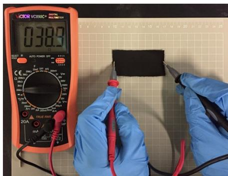
**Fig. S5** Photograph of the resistance measurement of the CCC by the multimeter.
