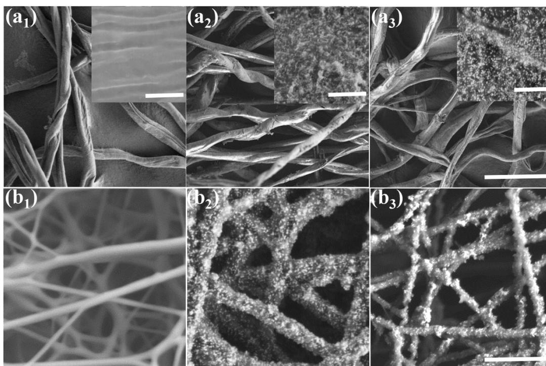
**Figure S7.** SEM images of original cotton (a<sub>1</sub>) and PLA fibers (b<sub>1</sub>), after coating with TA/Ag<sup>0</sup> (a<sub>2</sub>, b<sub>2</sub>) and TA-gold (a<sub>3</sub>, b<sub>3</sub>). The insets are the magnified images of corresponding samples. The scale bar is 100  $\mu\text{m}$  in a, 1  $\mu\text{m}$  in b, 500 nm in the insets of a.
