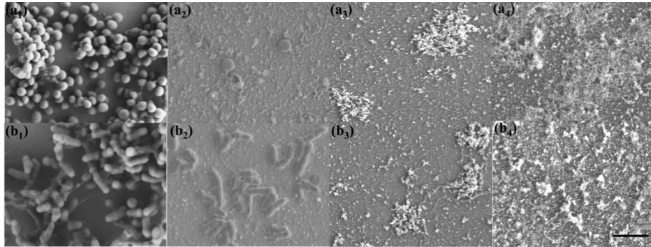
**Figure S8.** SEM images of (a) *S. aureus* and (b) *E. coli* after exposure to silica wafer (1 as control), TA/Ag coatings fabricated with different deposition time( 2, 3, 4 refer to 60s 300s and 300s-R3 respectively). The scale bar is 5  $\mu$ m.
