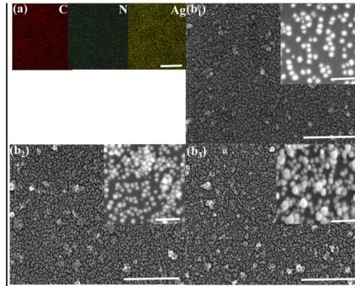
**Figure S3.** (a) EDS elemental mapping of TA/Ag coating. (b) SEM images of TA/Ag coatings on silicon with vortex time 10s ( $b_1$ ), 60s ( $b_2$ ) and 300s ( $b_3$ ). The scale bar is 200 nm in (a), 10  $\mu$ m in (b), 100 nm in the insets of (b).
