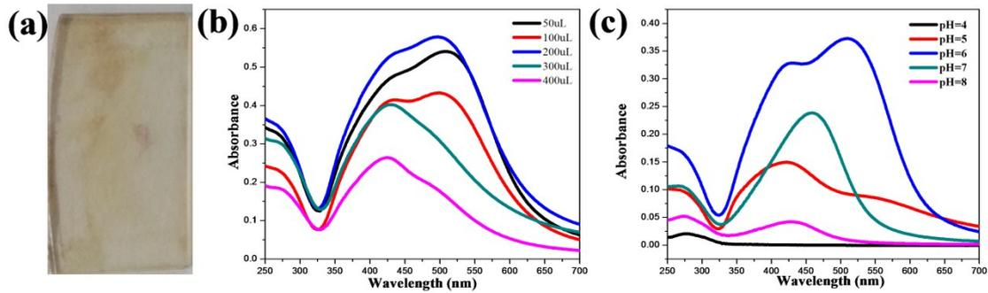
**Figure S4.** (a) The photo of TA/Ag coatings on quartz without PEI. (b) The UV-vis spectra of TA/Ag coatings with different amount of PEI. (c) The UV-vis spectra of TA/Ag coatings with different pH.
