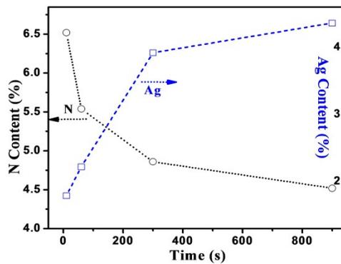
**Figure S5.** Dependence of nitrogen and silver content and on deposition time.
