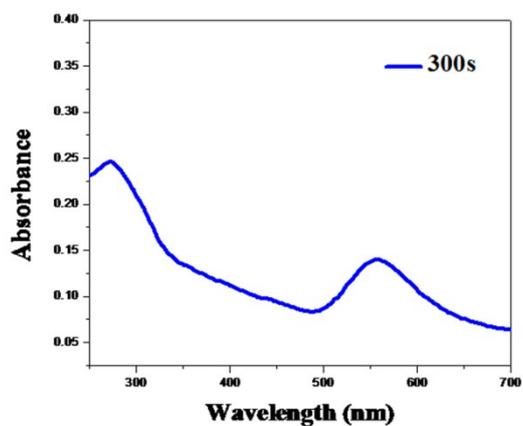
**Figure S6.** The UV-vis spectra of TA/Au coatings on quartz
