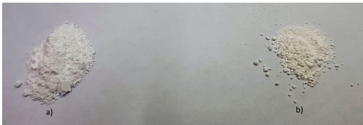
Figure S27. Photograph of MOF UiO-66 before (a) and after (b) heating at 280 °C for 30 minutes. A faint darkening of the MOF can be observed.
