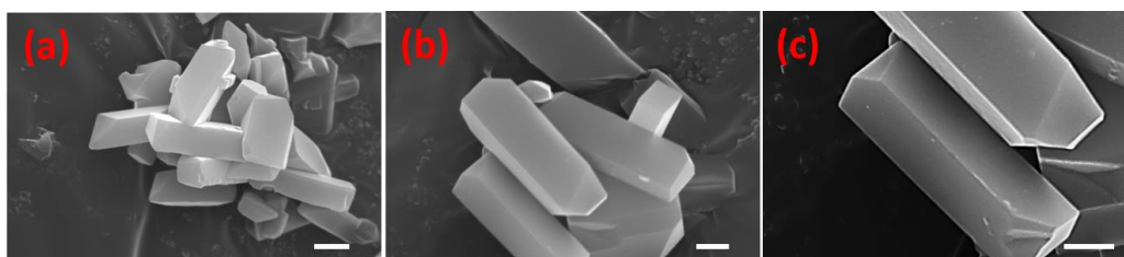
Figure S3. SEM images of cis -DMAAM crystals, [SDS] = 0.02 M, [1-dodecanol] = 0.0009 M, scale bar: (a) 2 \mu\text{m} , (b) 1 \mu\text{m} and (c) 1 \mu\text{m} .
