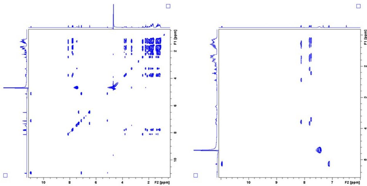
**Figure S42.** ROESY NMR [600 MHz, H<sub>2</sub>O/D<sub>2</sub>O 90:10] spectrum of compound 5
