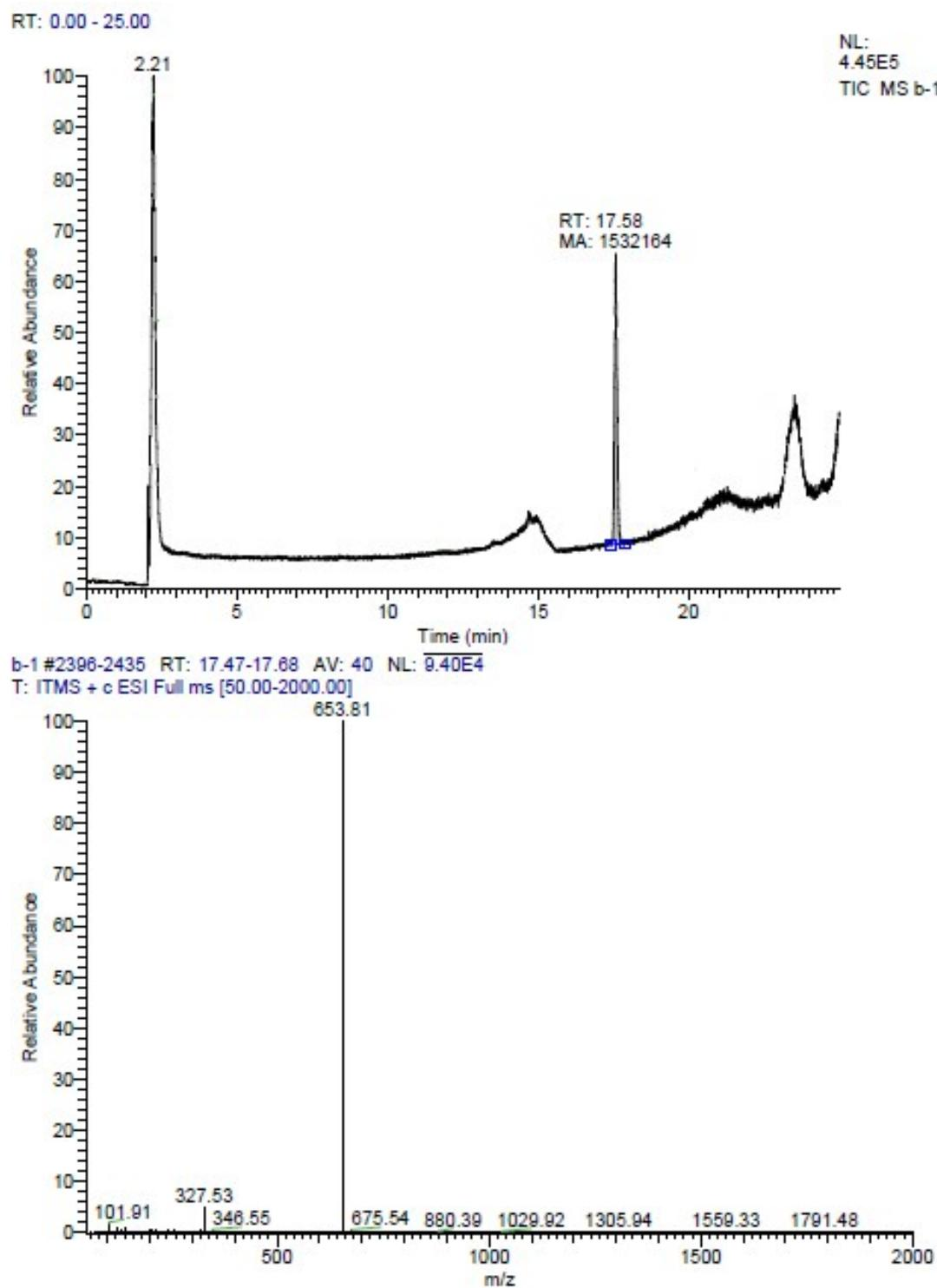
**Figure S67.** HPLC-MS chromatogram and mass spectrum of **2**: The following retention time and molecular weight were determined: **2**: {RT= 16.82, m/z = 655 [M + H]<sup>+</sup>}.
