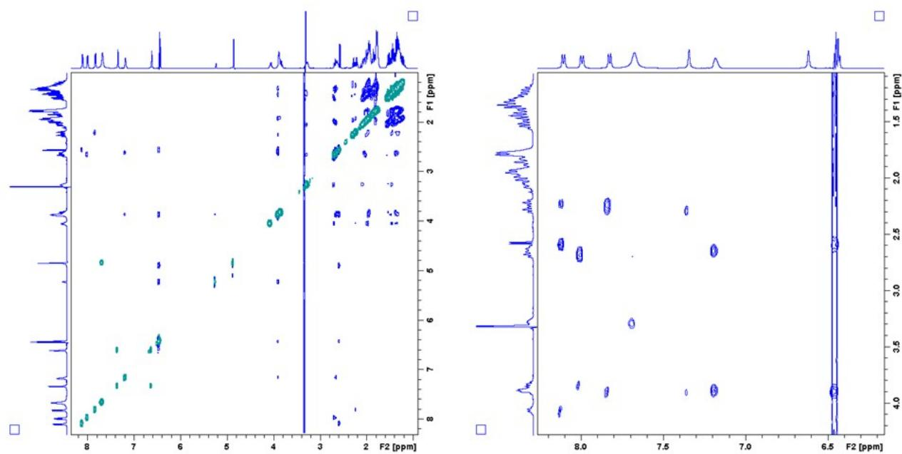
**Figure S37.** <sup>1</sup>H NMR [600 MHz, DMSO-d<sub>6</sub>] spectrum of compound 4
