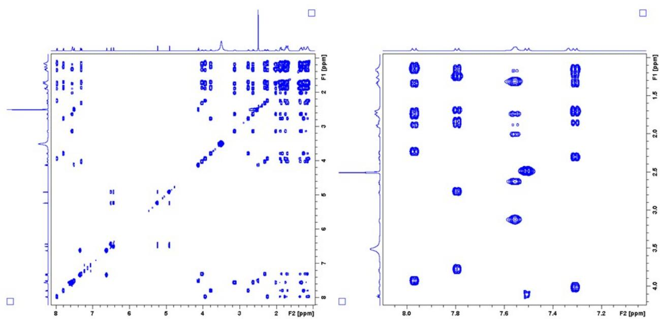
**Figure S21.** ROESY NMR [600 MHz, DMSO-*d*<sub>6</sub>) spectrum of compound 2
