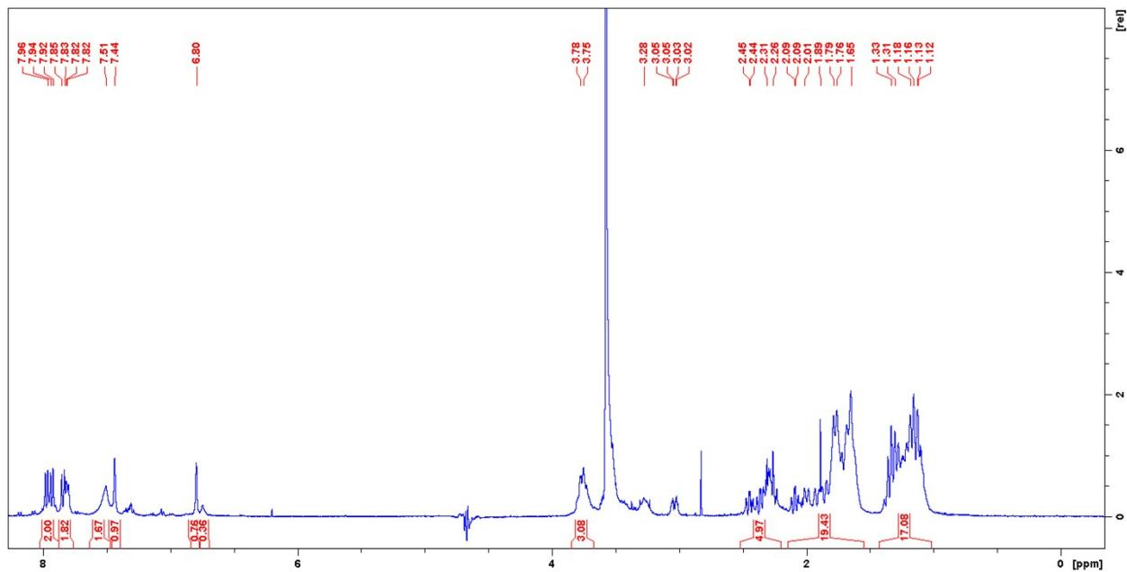
**Figure S50.** TOCSY NMR [500 MHz, H<sub>2</sub>O/D<sub>2</sub>O 90:10] spectrum of compound **6**
