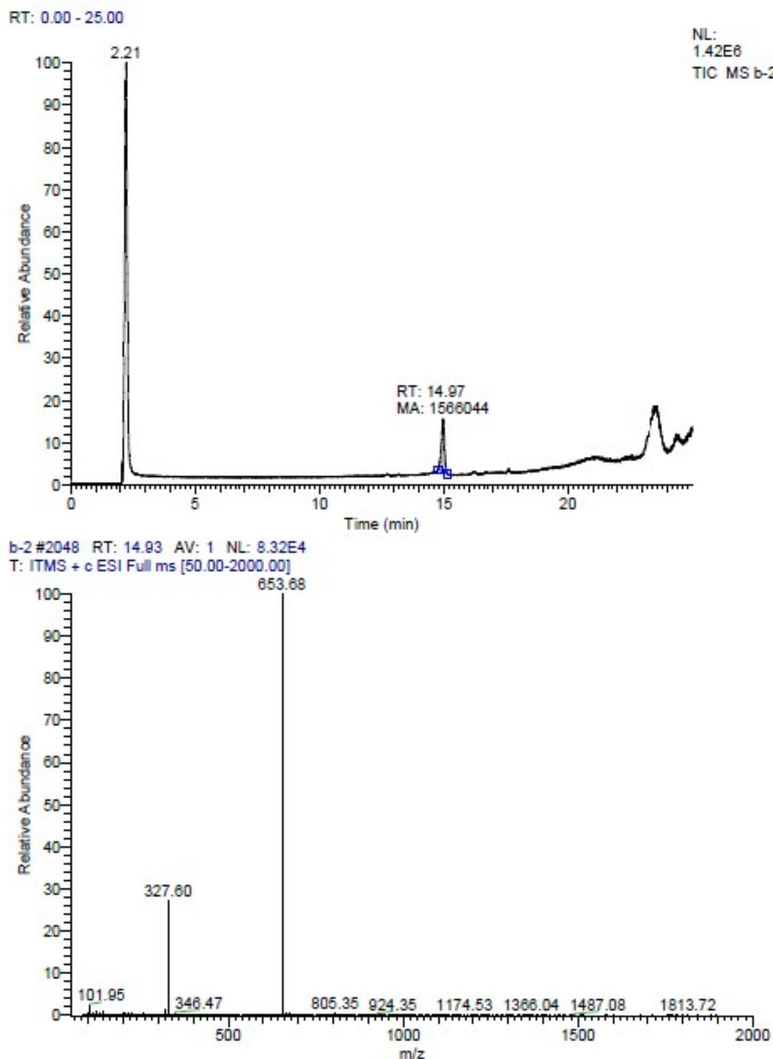
**Figure S69.** HPLC-MS chromatogram and mass spectrum of **4**: The following retention time and molecular weight were determined: **4**: {RT= 13.61, m/z = 655 [M + H]<sup>+</sup>}.
