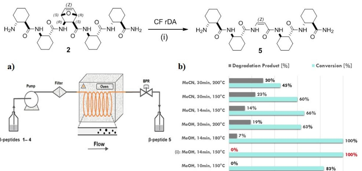
**Figure S1.** *Synthesis of oligomer 5: (a) illustration of CF rDA flow reactor; (b) reaction parameter optimization for the CF rDA reaction of **2**.*
