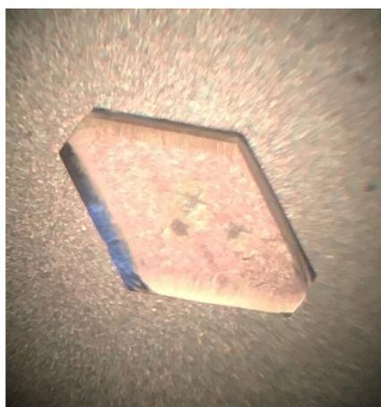
**Figure S2.** a) Observed theoretical morphology of LiPO<sub>2</sub>F<sub>2</sub>; (b) Photographic micrograph of LiPO<sub>2</sub>F<sub>2</sub> by spontaneous crystallization.
