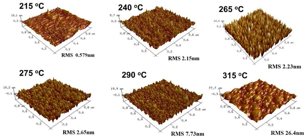
**Figure S3** AFM images of  $\text{Fe}_x\text{N}$  films deposited at varying temperatures using 6 s dose of  $\text{Fe}(\text{tBu-amd})_2$  and 0.6 s dose of  $\text{N}_2\text{H}_4$  by 500 cycles.
