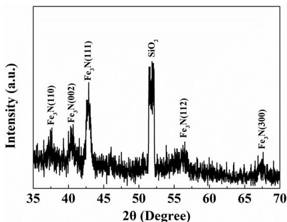
**Figure S5** XRD of  $\text{Fe}_x\text{N}$  films deposited at 290 °C using 6 s dose of  $\text{Fe}(\text{tBu-amd})_2$  and 0.6 s dose of  $\text{N}_2\text{H}_4$  by 500 cycles.
