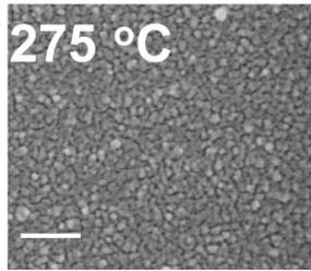
**Figure S2** SEM images of 500-cycle  $\text{Fe}_x\text{N}$  films deposited at 275 °C.
