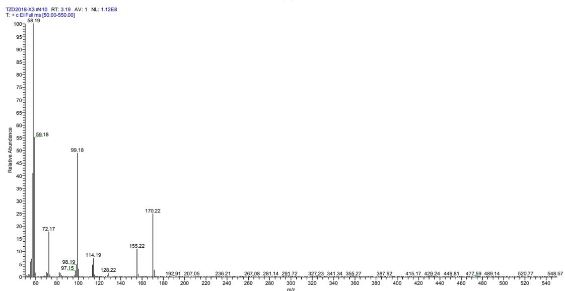
**Figure S7** GC-MS result of the pale yellow liquid which was trapped in the cold trap equipped between the ALD chamber and vacuum pump
