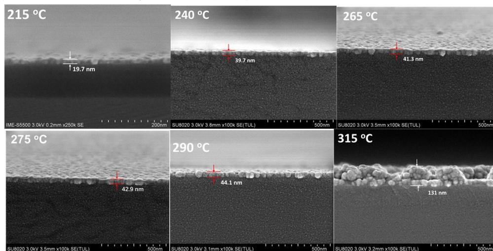
**Figure S1** Cross-sectional SEM images of  $\text{Fe}_x\text{N}$  films deposited at varying temperatures using 6 s dose of  $\text{Fe}(\text{tBu-amd})_2$  and 0.6 s dose of  $\text{N}_2\text{H}_4$  by 500 cycles.
