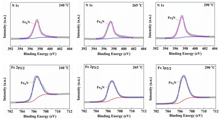
**Figure S4** N 1s and Fe  $2p_{3/2}$  XPS spectra of film deposited at ALD window
