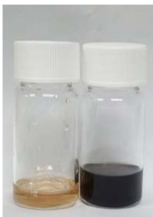
Figure s3: Electrolyte composed of 0.4 \text{ mol dm}^{-3} of \text{In}(\text{Tf}_2\text{N})_3 and 0.4 \text{ mol dm}^{-3} of \text{InCl}_3 in DME, before (left) and after (right) the measurement of a CV at room temperature on an gold disk electrode with a scan rate of 5 \text{ mV s}^{-1} .
