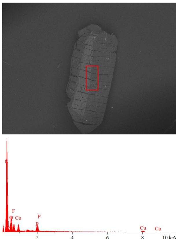
Fig. S10: the SEM surface analysis of Cu I -NDI and the EDX analysis of the elemental distribution.
