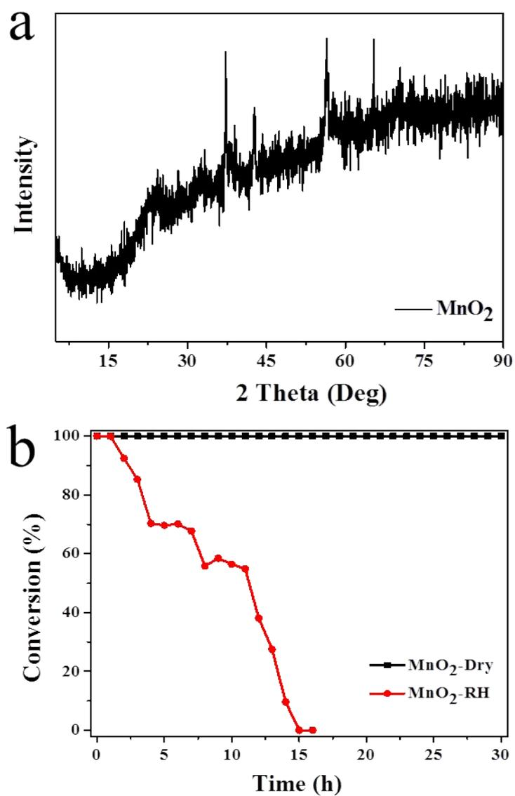
Figure S4 (a) The XRD patterns of referenced MnO<sub>2</sub> (b) Ozone catalytic decomposition over referenced MnO<sub>2</sub> at room temperature in dry air and at high relative humidity (RH~90%) with an ozone concentration of 20 ppm.
