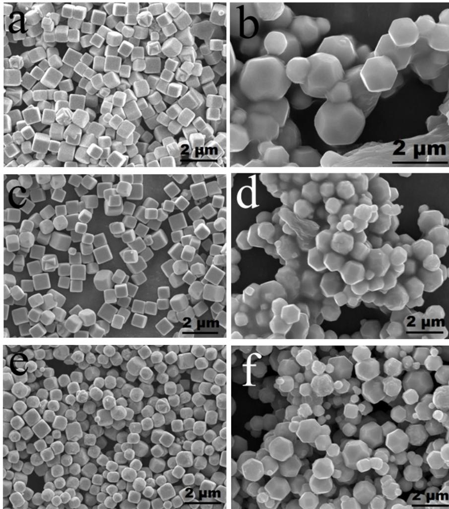
Figure S3 (a,c,e) SEM of samples collected at 1 h, 3 h and 6 h reduced by ascorbic acid (b,d,f) SEM of samples collected at 1 h, 3h and 6 h reduced by glucose.
