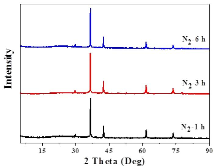
Figure S1 The XRD patterns of samples obtained at different reaction time under N<sub>2</sub> atmosphere.
