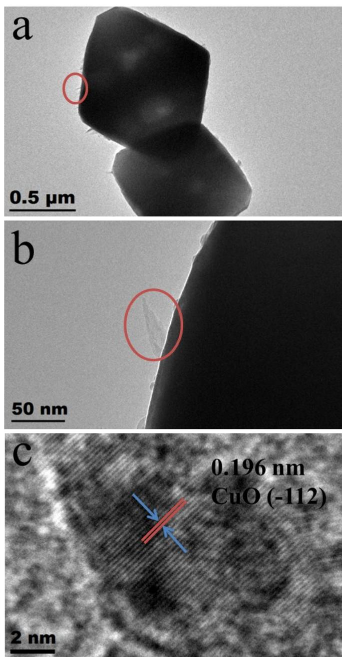
Figure S2 (a-b) TEM and (c) HRTEM of sample obtained at 6 h under N<sub>2</sub> atmosphere.
