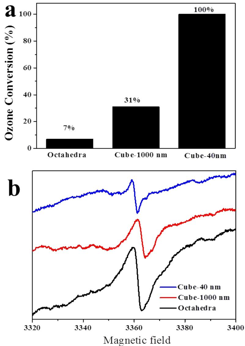
Figure S5 (a) ozone conversion after 2 h test of octahedra, cube-1000 nm and cube-40 nm  $\text{Cu}_2\text{O}$  (Ozone inlet concentration: 20 ppm for octahedra and cube-1000 nm, 200 ppm for cube-40nm,  $T=25\text{ }^\circ\text{C}$ ,  $SV= 60,000\text{ mL g}^{-1}\text{ h}^{-1}$ ) (b) EPR spectra of octahedra, cube-1000 nm and cube-40 nm.
