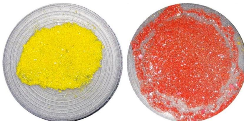
Figure S10: Optical microscope image of PU-1 crystal: as-synthesized(left), water treatment(right)
