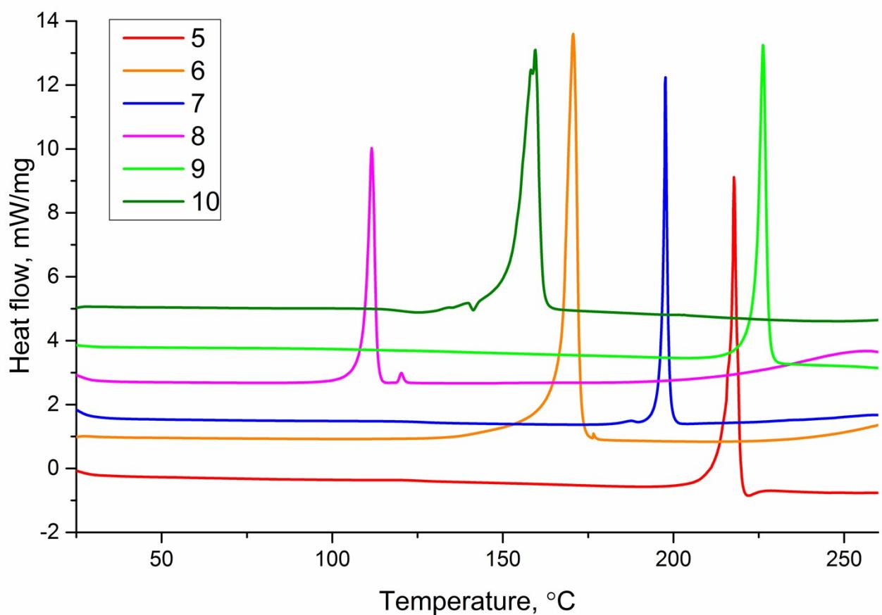
**Figure 3SI.** DSC curves of compounds **5-10** recorded at  $10 \text{ K}\cdot\text{min}^{-1}$ .
