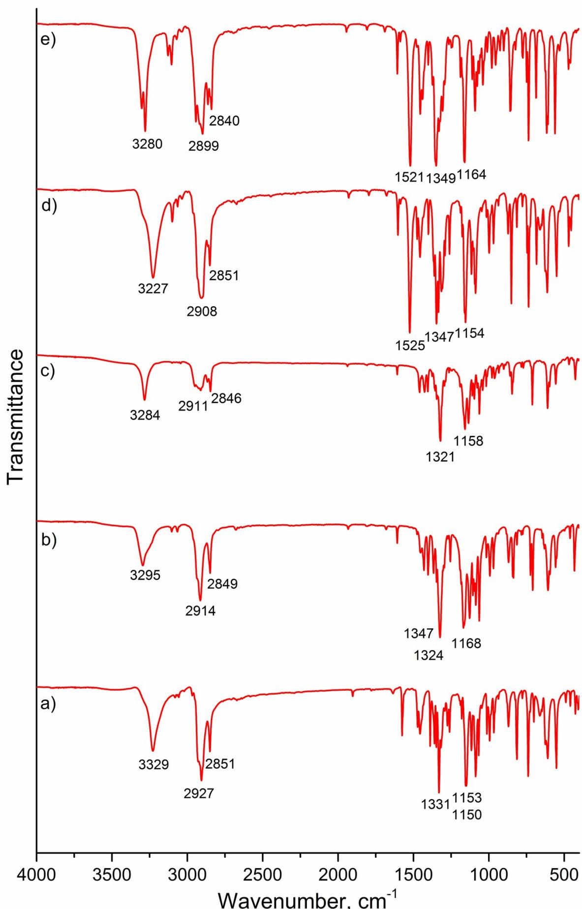
Figure 4SI. IR spectra for compounds **5** (a), **7** (b), **8** (c), **9** (d) and **10** (e)
