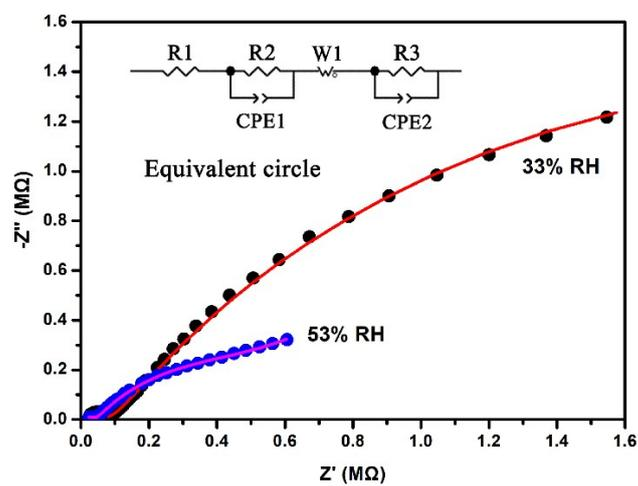
Fig. S4 Nyquist plots of Compound 1 at 30 °C and 33% RH (black) and at 30 °C and 53% RH (blue) and their equivalent electrical-circuit fitting lines (red for 33% RH and pink for 53% RH).
