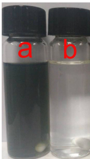
Fig. S3 The photograph of \text{Cu}_{2-x}\text{Se} methanol dispersion before (a) and after (b) addition of TBP in air.
