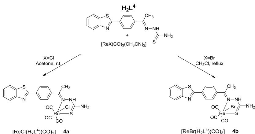
Scheme S8. Synthesis of the complexes with H<sub>2</sub>L<sup>4</sup>.
