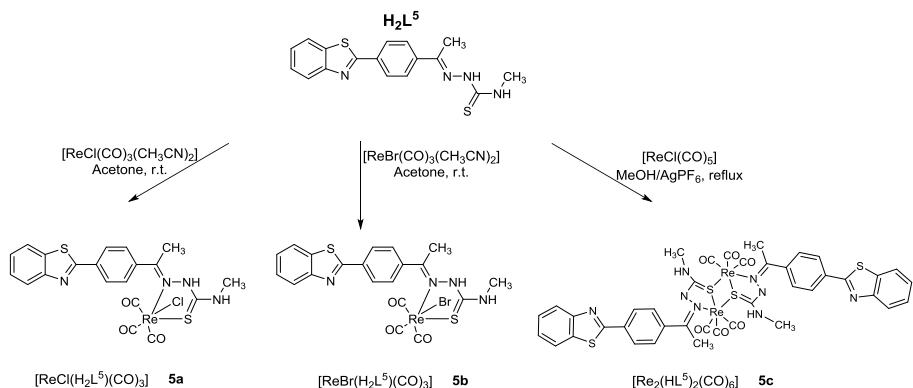
Scheme S9. Synthesis of the complexes with  $H_2L^5$ .
