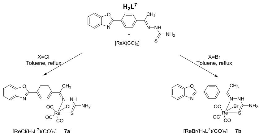
Scheme S11. Synthesis of the complexes with  $\text{H}_2\text{L}^7$ .
