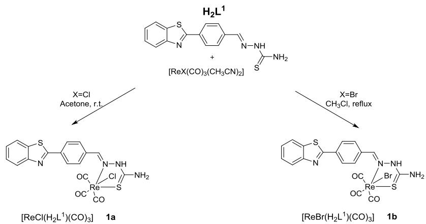
Scheme S5. Synthesis of the complexes with H<sub>2</sub>L<sup>1</sup>.
