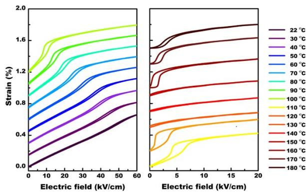
**Fig. S4** Unipolar strain-electric field loops for [100]-oriented Mn:PIN-PMN-PT single crystals at various temperatures.
