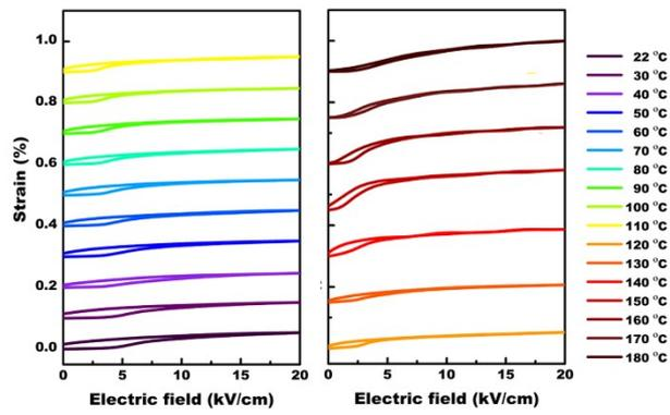
**Fig. S6** Unipolar strain-electric field loops for [111]-oriented Mn:PIN-PMN-PT single crystals at various temperatures.
