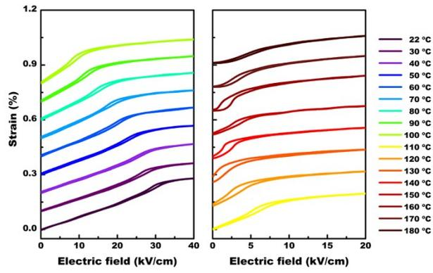
**Fig. S5** Unipolar strain-electric field loops for [110]-oriented Mn:PIN-PMN-PT single crystals at various temperatures.
