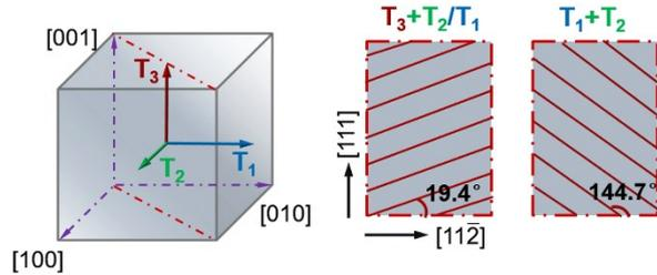
**Fig. S3** Permissible domain configurations and the 90° domain patterns at 140 °C in [111]-oriented Mn:PIN-PMN-PT single crystals with 3T engineered domain configuration. The traces of the domain walls on  $(\bar{1}10)$  planes form 19.4° or 144.7° angles with respect to  $[11\bar{2}]$ .
