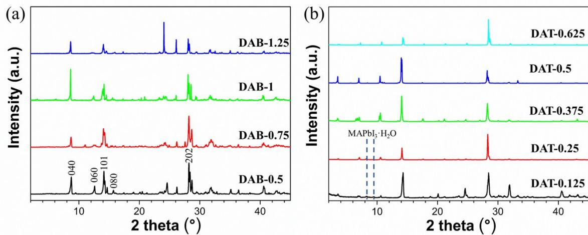
**Figure S1.** XRD patterns of (a) **DAB** samples synthesized with DAB added by 0.5, 0.75, 1, 1.25 times of the stoichiometric amount of  $\text{DAB}(\text{MA})_2\text{Pb}_3\text{I}_{10}$  and (b) **DAT** samples synthesized with DAT added by 0.125, 0.25, 0.375, 0.5 and 0.625 times of the stoichiometric amount of  $\text{DAT}(\text{MA})_2\text{Pb}_3\text{I}_{10}$ .
