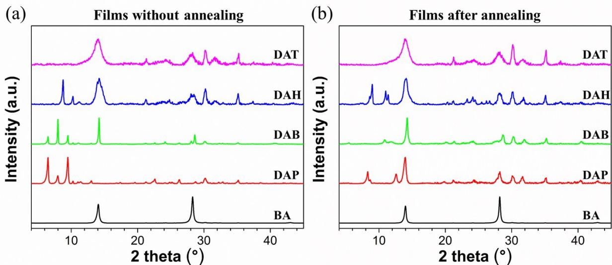
**Figure S2.** XRD patterns of **BA** and **DAX** films (a) without annealing and (b) after annealing.
