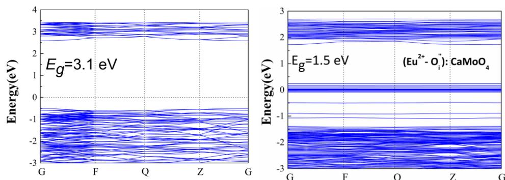
Figure S3: The Band structure of pure CaMoO<sub>4</sub> and the (Eu<sup>2+</sup>-O<sub>i</sub><sup>2-</sup>):CaMoO<sub>4</sub>.
