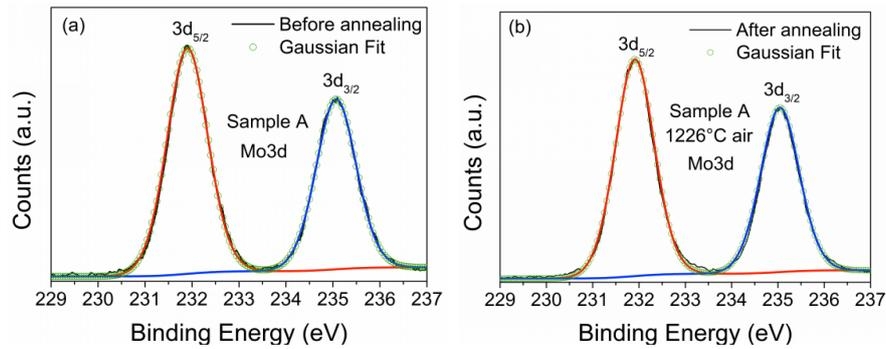
Figure S5: The Mo3d XPS of sample A before (a) and after (b) annealing in air atmosphere.
