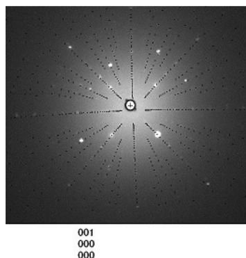
Figure S2: The good quality of 0.01 at.%  $\text{Eu}^{3+}$ : $\text{CaMoO}_4$  SCF tested by the X-ray Laue diffractometer.
