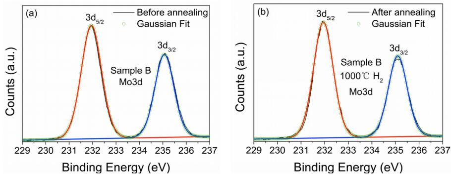
Figure S6: The Mo3d XPS of sample B before (a) and after (b) annealing in  $\text{H}_2$  atmosphere.
