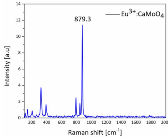
Figure S4: The Raman spectrum of the  $\text{Eu}^{3+}:\text{CaMoO}_4$  SCF sample
