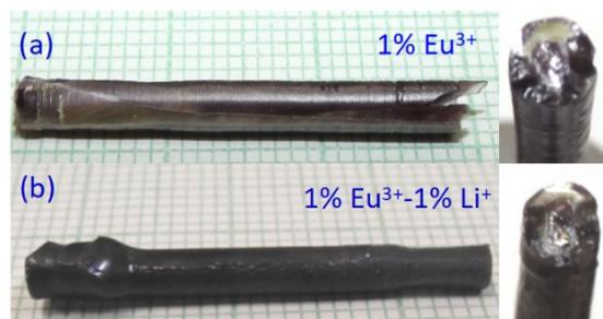
Figure S1: Two SCFs of  $\text{CaMoO}_4$ : 1%  $\text{Eu}^{3+}$  (a) and 1%  $\text{Eu}^{3+}$ -1%  $\text{Li}^+$  (b) grown with a Pt wire in air atmosphere.
