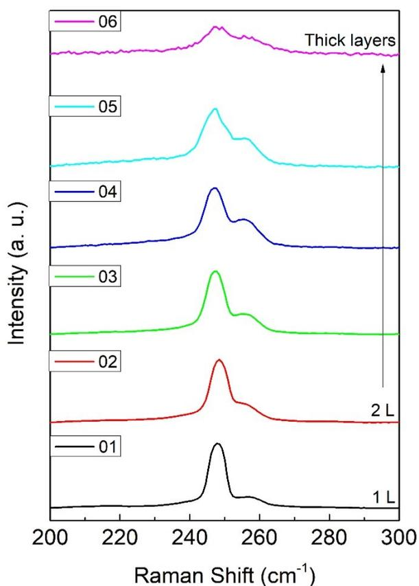
Fig. S2 Raman spectra collected from the regions of the 2D WSe<sub>2</sub> with different thickness shown in Fig. S1.
