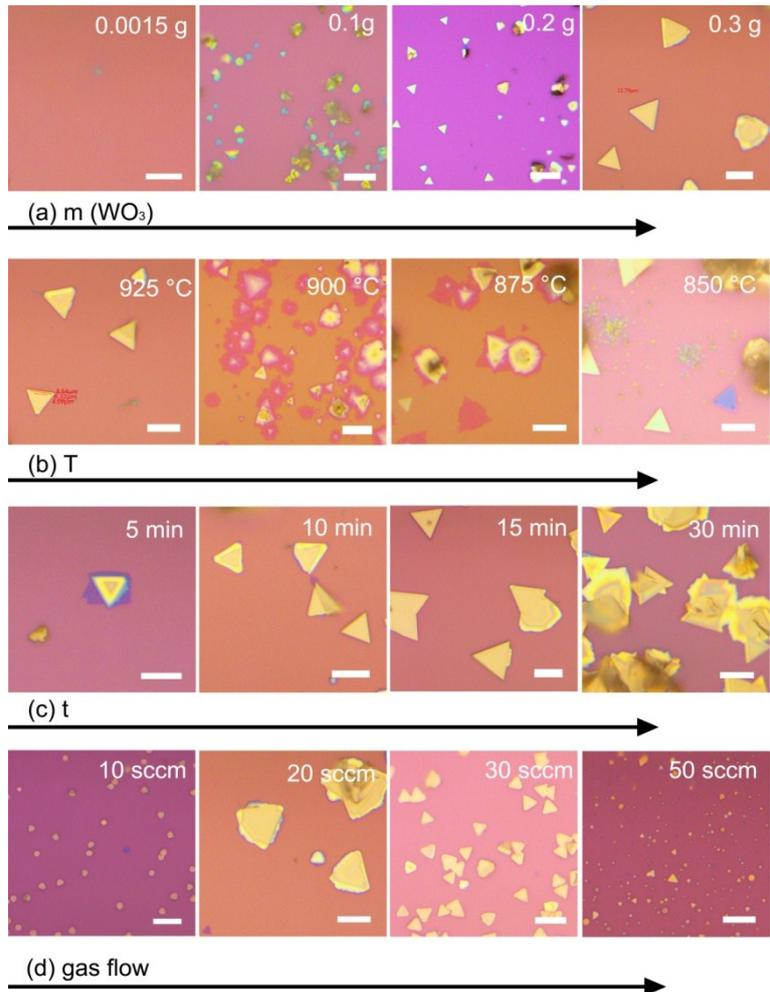
Fig. S6 OM image of 2D WSe<sub>2</sub> flakes grown by CVD without NaCl. Optimized parameters: (a) mass (WO<sub>3</sub>); (b) reaction temperature T; (c) reaction time t; and (d) gas flow. Scale bars, 10 μm.
