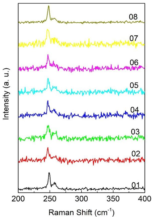
Fig. S8 Raman spectra collected from the regions of a WSe<sub>2</sub> flake with a spiral dislocation shown in Fig. 4(c).
