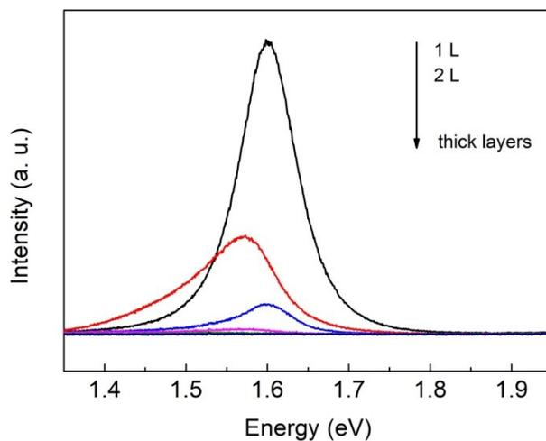
Fig. S4 PL spectra collected from the regions of the 2D WSe<sub>2</sub> with different thickness shown in Fig. S1.
