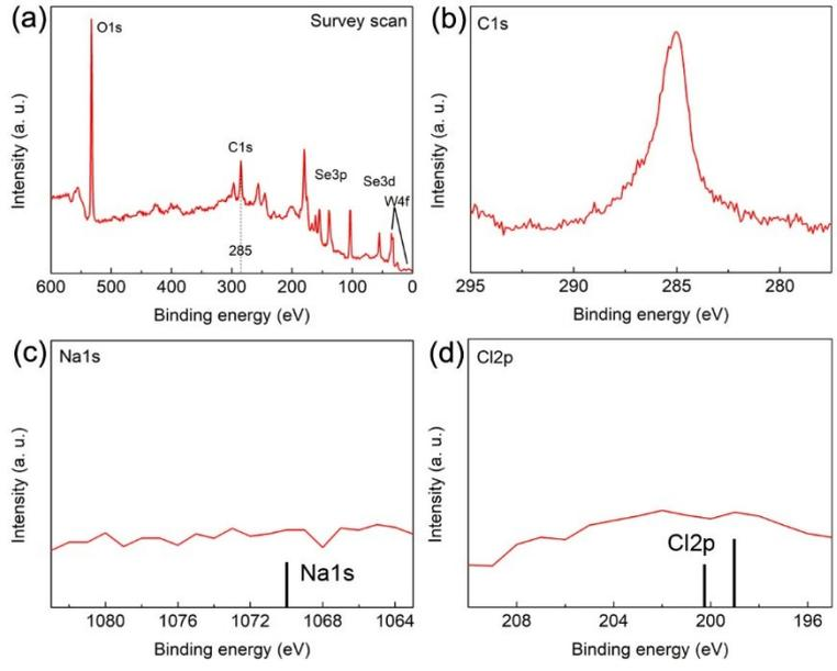
Fig. S5 XPS spectra of the as-grown 2D WSe<sub>2</sub>. (a) survey scan, (b) C1s, (c) Na1s, and (d) Cl2p.
