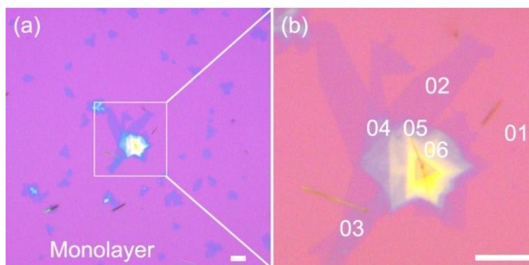
Fig. S1 OM images showing the coexistence of monolayer, bilayer and multilayers in the WSe<sub>2</sub> flakes. (a) overview. (b) zoom-in of (a). Scale bars, 10  $\mu\text{m}$ .
