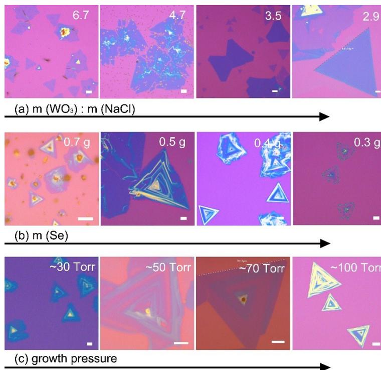
Fig. S7 OM image of 2D WSe<sub>2</sub> flakes grown by CVD with NaCl. Optimized parameters: (a) mass (WO<sub>3</sub>) : mass (NaCl); (b) mass (Se); (c) growth pressure. Scale bars, 10 μm.
