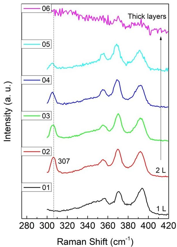
Fig. S3 Raman spectra collected from the regions of the 2D WSe<sub>2</sub> with different thickness shown in Fig. S1.
