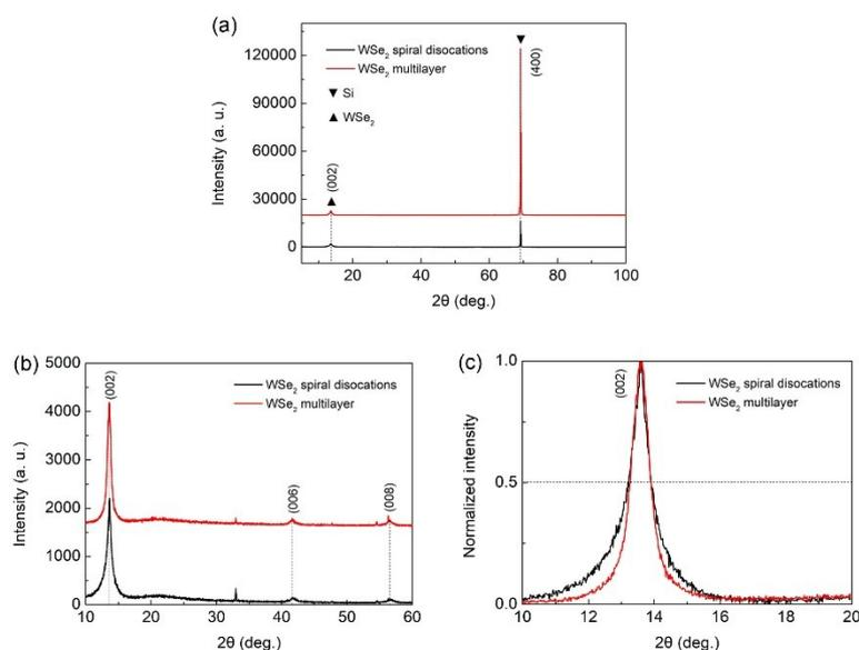
Fig. S10 XRD patterns from the WSe<sub>2</sub> spiral dislocation and WSe<sub>2</sub> multilayer. (a) XRD patterns of WSe<sub>2</sub> and Si substrate. (b) XRD patterns of WSe<sub>2</sub>. (c) Normalized intensities of the (002) diffraction peaks, respectively.
