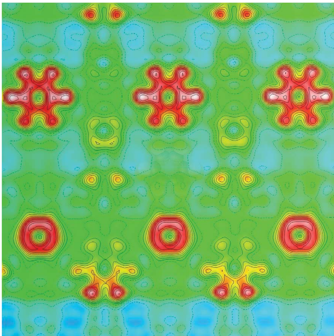
Fig. S20. Fourier map of the observed electron density of \text{C}_6\text{H}_6:\text{C}_6\text{F}_6 phase II calculated from |\mathbf{F}(\text{obs})| and phase \phi of \mathbf{F}(\text{calc}) taken across a slice of the unit cell showing the smeared out density of the C atoms of the \text{C}_6\text{H}_6 molecule due to its dynamics plus position of the \text{C}_6\text{F}_6 molecule. The motion is attributed to stochastic jump rotations about the molecular six-fold axis.
