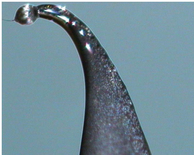
Fig. S6. \text{C}_6\text{H}_6:\text{C}_6\text{F}_6 was filled in a 0.5 mm capillary, flame sealed, and the sample was then condensed at the sealed end and allowed to anneal for 4 days on a twin-source Agilent SuperNova diffractometer equipped with a micro-focus Cu X-ray beam (50 kV, 0.8 mA) and an Atlas (135 mm CCD) detector. The sample temperature was held at 290 K, just below the melting point at 298 K, with an Oxford Instruments Cryojet5 ® to facilitate crystal growth. It was important to check that the capillary is 100% sealed to prevent loss of sample when kept at room temperature over many days.
