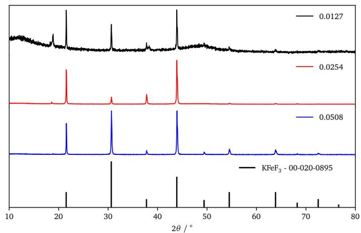
**Figure S4** XRD patterns showing the co-thermolysis product,  $\text{KFeF}_3$ , at different molar concentrations of iron precursor in the reaction mixture ( $\frac{Fe}{OA+OM}$ ). The precursor stoichiometry ( $\frac{K}{Fe}$ ) was kept constant during these experiments.
