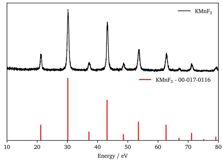
Figure S5 XRD pattern of hot-injection product,  $\text{KMnF}_3$
