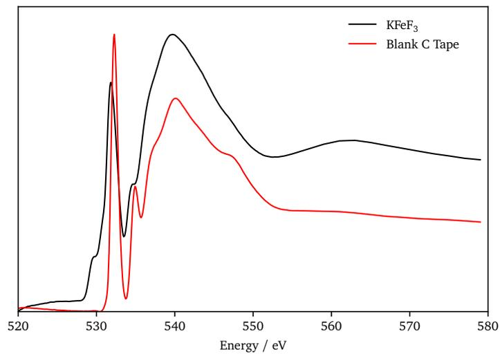
**Figure S8** Soft x-ray absorption spectroscopy (XAS) spectra (total electron yield (TEY) signal) showing similar patterns between  $\text{KFeF}_3$  (black) and carbon tape substrate (red) oxygen  $K$ -edge data.
