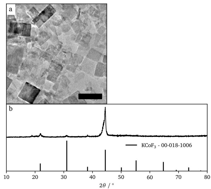
Figure S6 TEM image and XRD pattern of hot-injection product,  $\text{KCoF}_3$ , with stoichiometric ratio  $\frac{K}{Co}=3.00$ . Scale bar represents 50 nm
