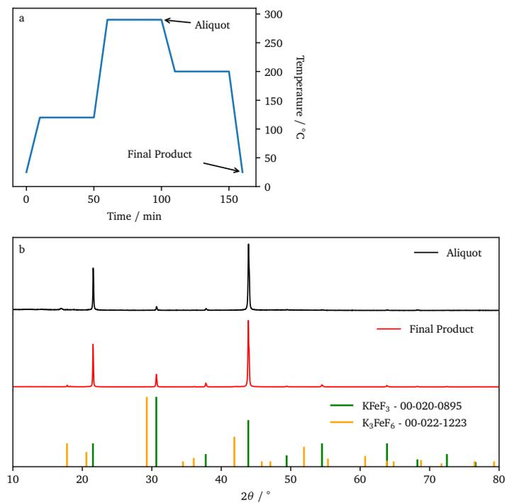
**Figure S1** Temperature profile of the experiment denoting where the aliquot and final product were collected (a), and powder x-ray diffraction (XRD) patterns showing the composition of these products (b).
