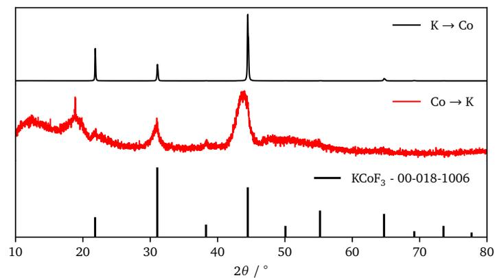
**Figure S7** XRD patterns of hot-injection product,  $\text{KCoF}_3$ , with varying the mobile and static hot-injection solutions.
