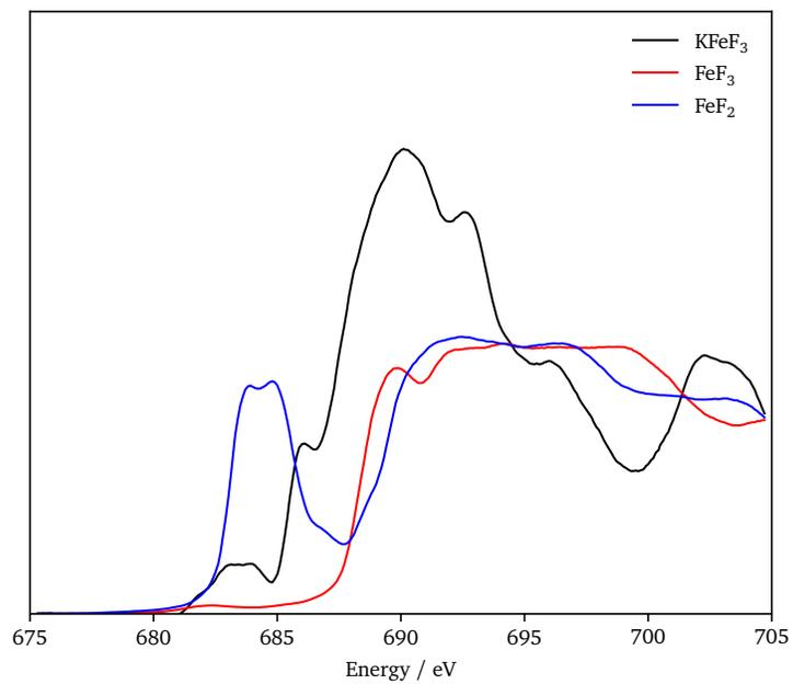
**Figure S10** F K-edge data (total fluorescence yield (TFY)) of KFeF<sub>3</sub> (black), FeF<sub>3</sub> (red), and FeF<sub>2</sub> (blue) taken at the same beamline (4-ID-C, Advanced Photon Source, Argonne National Laboratory.)
