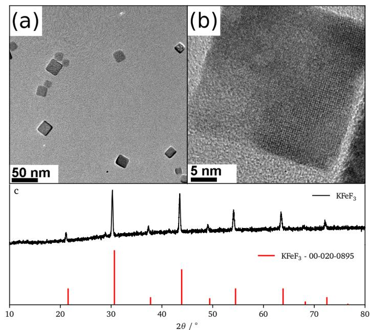
**Figure S3** Transmission electron microscopy (TEM) images (a and b) and XRD spectra (c) of  $\text{KFeF}_3$  nanocrystals synthesized from a double fluorine source method.
