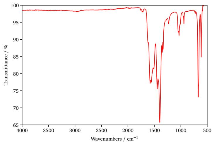
**Figure S2** Infrared (IR) spectroscopy of  $\text{Fe}(\text{CH}_3\text{COO})_2$  precursor.
