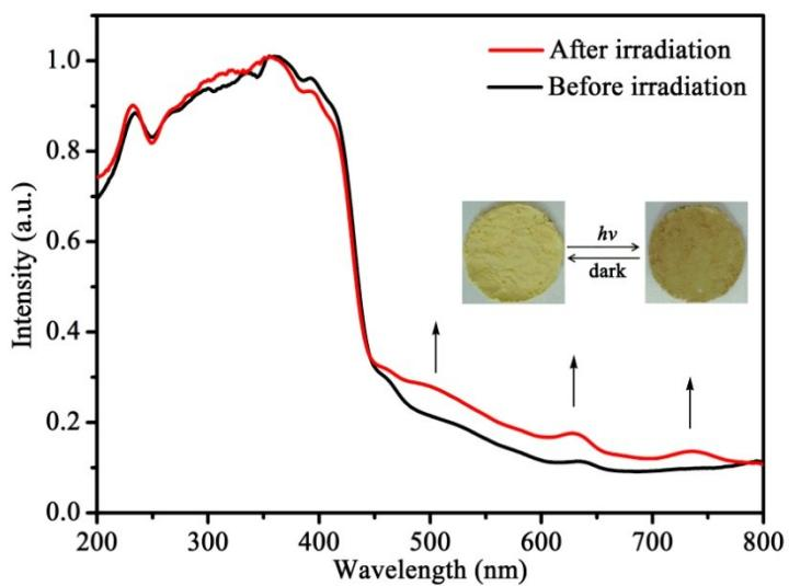
**Fig. S5** UV-Vis spectrum of DPMNI free ligand before and after irradiation by 300W xenon lamp.
