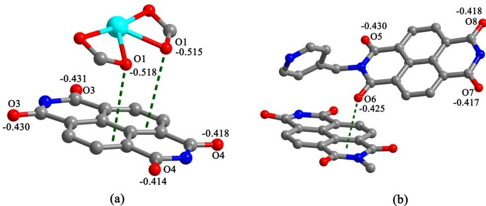
**Fig. S10** The charge of different O atoms in two kinds lone pair- $\pi$  interactions as electron transfer pathways in compounds **1** (a)-**2** (b).
