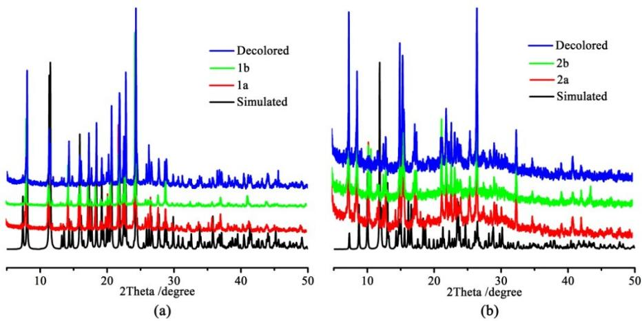
**Fig. S7** PXRD patterns of compounds **1** (a) and **2** (b). Lables: **1a**, **2a**: before irradiation; **1b**, **2b**: after irradiation; **Decolored**: by dark treatment about one month; **Simulated**: according to their single-crystal X-ray diffraction data.
