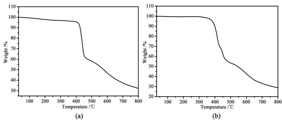
**Fig. S9** TGA curves of compounds **1** (a) and **2** (b) were carried out in powder states under N<sub>2</sub> atmosphere.
