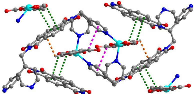
**Fig. S2** The interactions (green: lone pair-π interactions; orange and pink: CH-π interactions) between different molecules from 2D networks forming 3D supramolecular structure in compound **1**.
