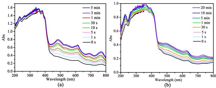
**Fig. S4** Time-dependent UV-Vis spectra of compounds **1** (a) and **2** (b) upon irradiation by 300W xenon lamp.
