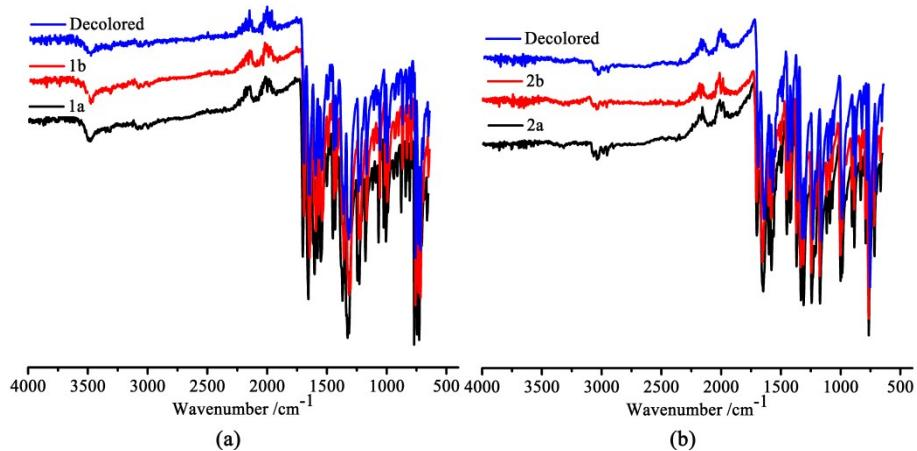
**Fig. S8** IR spectra of compounds **1** (a) and **2** (b). Lables: **1a**, **2a**: before irradiation; **1b**, **2b**: after irradiation; **Decolored**: by dark treatment about one month;
