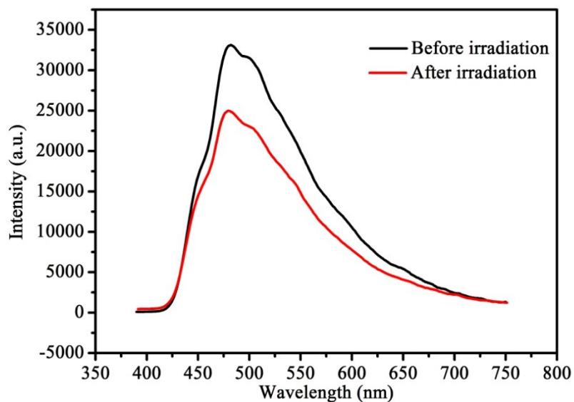
**Fig. S6** Luminescence spectrum of DPMNI free ligand before and after irradiation by 300W xenon lamp.
