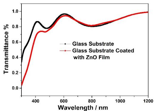
**Fig. S6** Simulated result of transmittance using finite difference time domain method.
