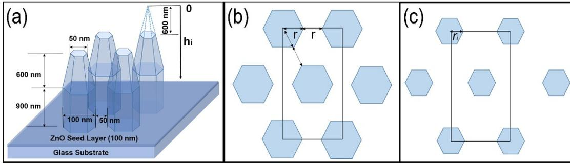
**Fig. S8** Correlation model parameters for effective refractive index simulation. (a) The size parameters and coordinate axis; (b) the radius and area of unit cell; and (c) the radius and area of the slice cross section at the height of  $h_i$ .
