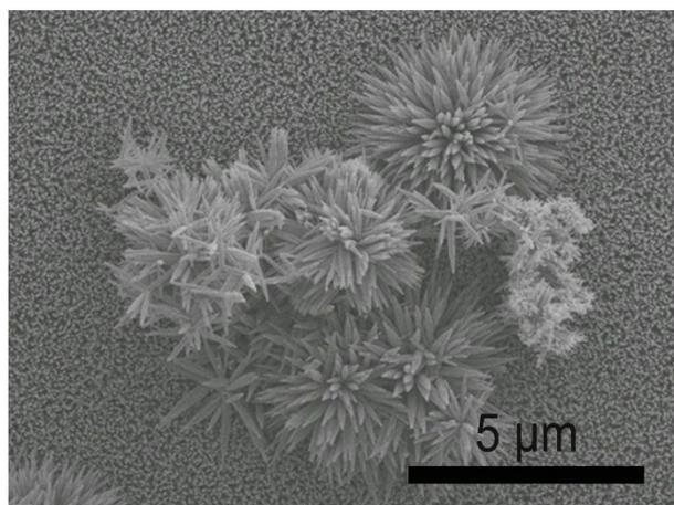
**Fig. S3** The result of microflowers local depositing on the top of nanopike arrays.
