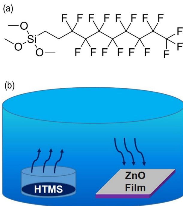
**Fig. S2** Low surface modification of ZnO film by HTMS. (a) The molecular structure of HTMS; and (b) the modification process.
