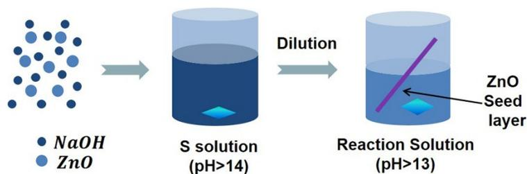
**Fig. S1** Reaction diagram using a diluent hydrolysis approach.
