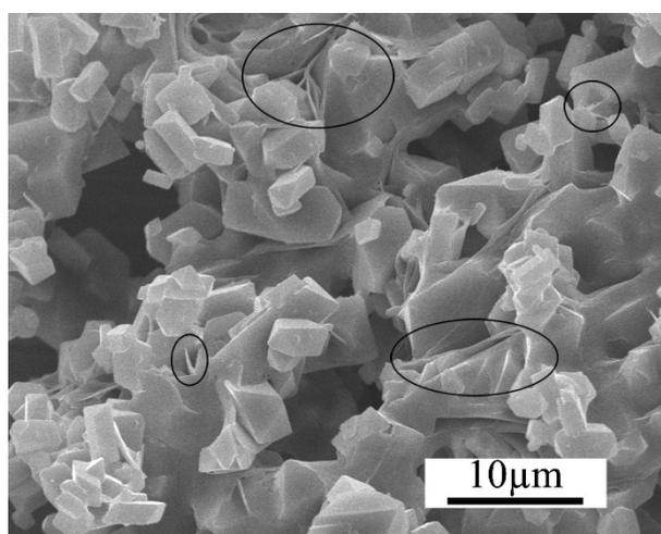
**Fig. S5** The result of ZnO growth on glass substrate, with 20 dilution ratio in room temperature environment.
