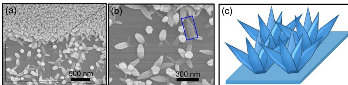
**Fig. S4** The result of ZnO growth on glass substrate, with 20 dilution ratio in 60 °C environment. (a) Low magnification SEM image; (b) low magnification SEM image; and (c) schematic diagram of ZnO cluster composed of nanospikes.
