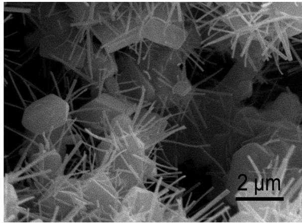
**Fig. S9** The result of ZnO growth in 20 dilution ratio diluent, in room temperature environment for 15 min.
