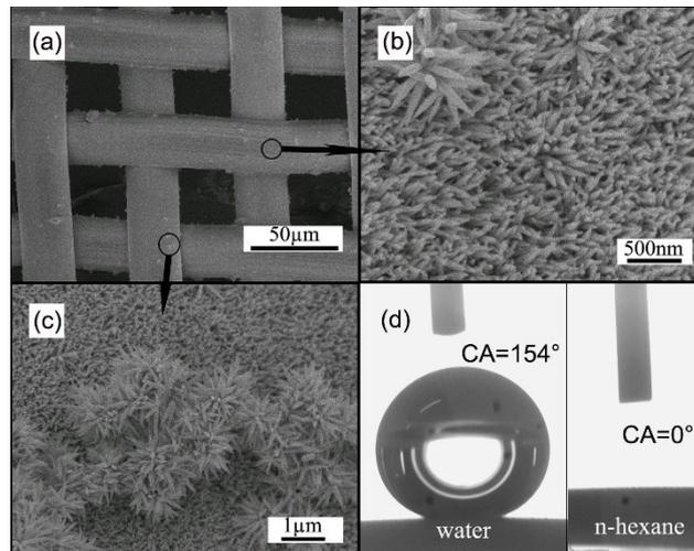
**Fig. S10** The surface morphology and the wettability on copper grid using saturated solution diluent hydrothermal reaction method. (a) The low magnification of the grid; (b) and (c) the ZnO nanorods and microclusters growing on the stainless steel wire; and (d) the wettability of water and n-hexane on the surface modified by HTMS.
