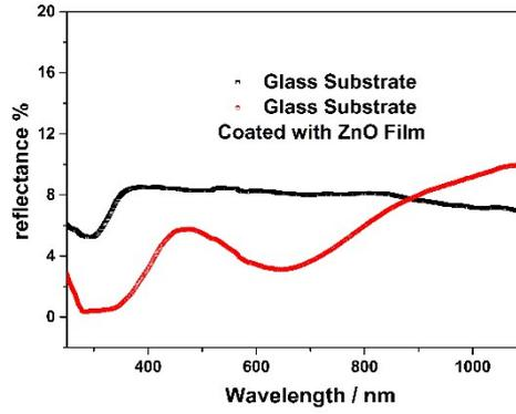
**Fig. S7** The reflectance result of the glass substrate and ZnO nanopikes coated glass.
