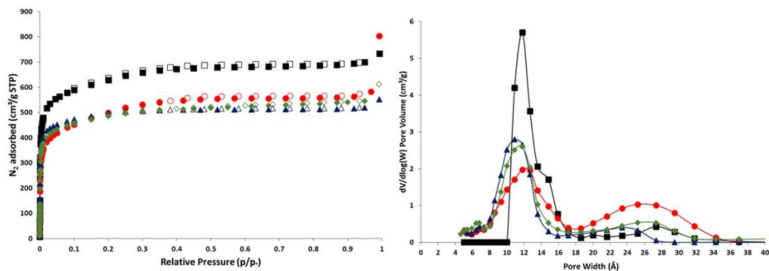
**Figure S13.**  $N_2$  isotherms (left) and pore size distribution (right) of NU-901-HCl (black squares), NU-901-SALI-isonic (red circles), NU-901-SALI-nico (blue triangles), and NU-901-SALI-BA-3,5-NH<sub>2</sub> (green diamonds). Adsorption = filled, desorption = empty markers.
