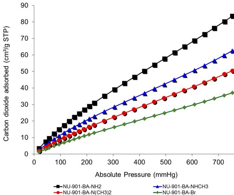
**Figure S23.** CO<sub>2</sub> adsorption curves of NU-901-BA-NH<sub>2</sub> (black squares), NU-901-BANHCH<sub>3</sub> (blue triangles), NU-901-BA-N(CH<sub>3</sub>)<sub>2</sub> (red circles), and NU-901-BA-Br at 273K.
