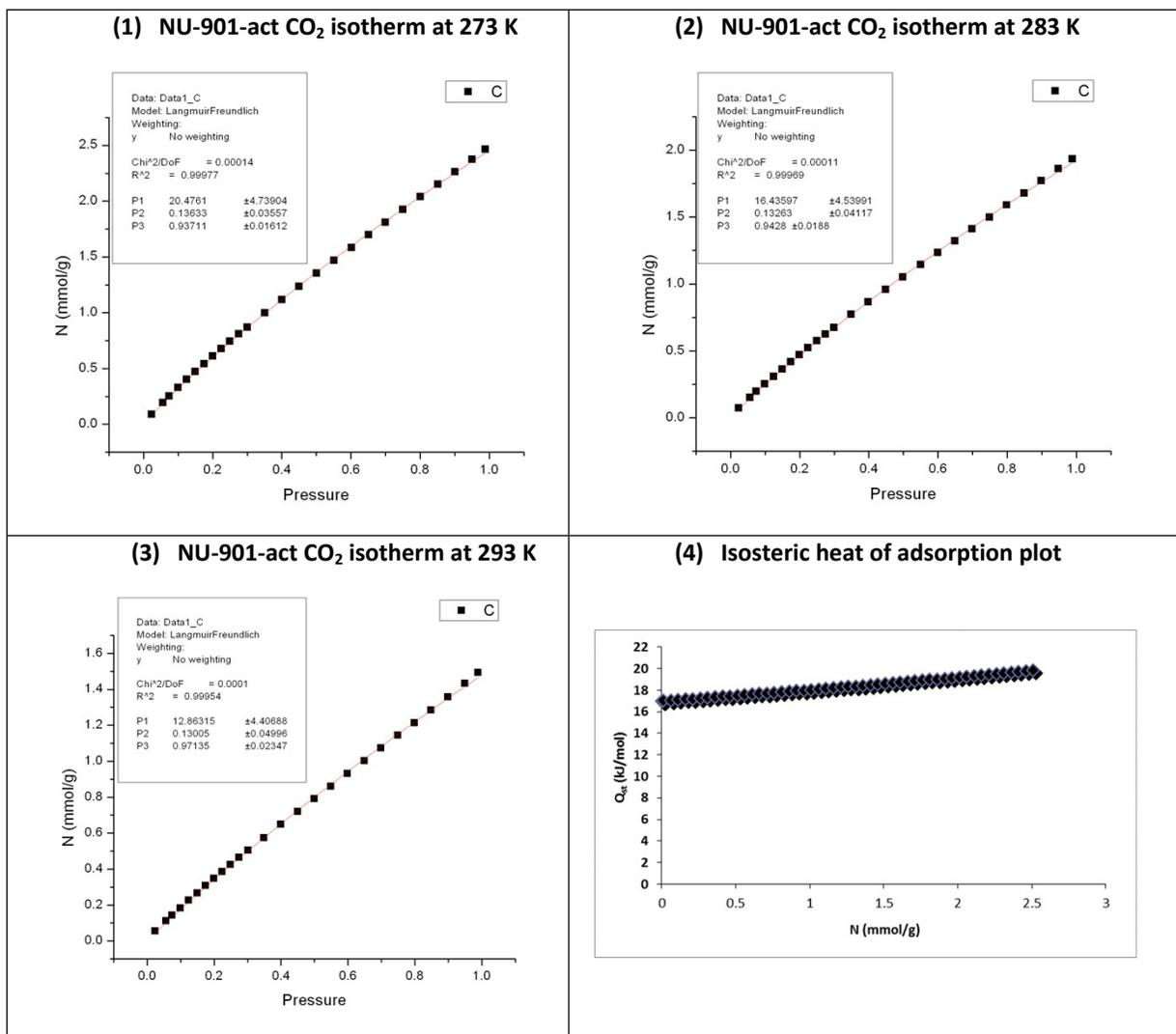
**Figure S21.** CO<sub>2</sub> adsorption curves, fitting and parameters for NU-901-act at 273 K (1), 283 K (2), 293 K (3), and isosteric heat of adsorption ( $Q_{st}$ ) calculated by the single-site Langmuir-Freundlich model (4).
