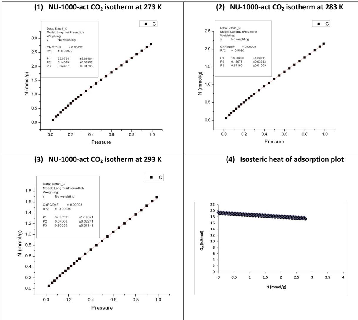
**Figure S19.** CO<sub>2</sub> adsorption curves, fitting and parameters for NU-1000-act at 273 K (1), 283 K (2), 293 K (3), and isosteric heat of adsorption ( $Q_{st}$ ) calculated by the single-site Langmuir-Freundlich model (4).
