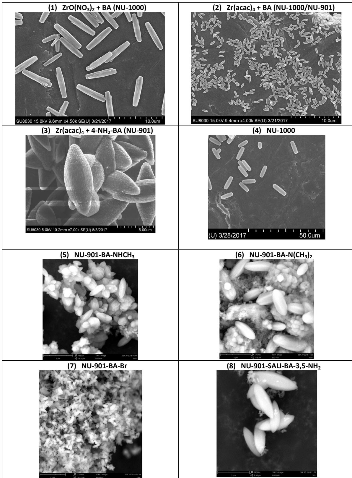
**Figure S17.** SEM images of MOF synthesized with  $\text{ZrO}(\text{NO}_3)_2$  (1),  $\text{Zr}(\text{acac})_4 + \text{BA}$  (2),  $\text{Zr}(\text{acac})_4 + 4\text{-NH}_2\text{-BA}$  (3), NU-1000 (4), NU-901-BA-NHCH<sub>3</sub> (5), NU-901-BA-N(CH<sub>3</sub>)<sub>2</sub> (6), NU-901-BA-Br (7), and NU-901-SALI-BA-3,5-NH<sub>2</sub> (8).
