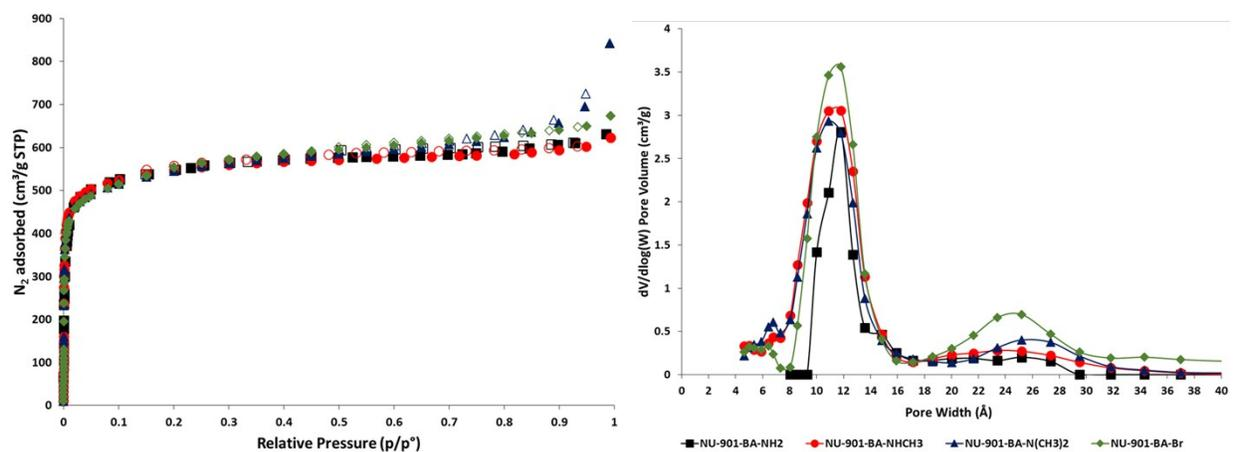
**Figure S12.**  $N_2$  isotherms of NU-901-BA-NH<sub>2</sub> (black squares), NU-901-BA-NHCH<sub>3</sub> (red circles), NU-901-BA-N(CH<sub>3</sub>)<sub>2</sub> (blue triangles), and NU-901-BA-Br (green diamonds) synthesized through *de novo* MOF synthesis. Adsorption = filled, desorption = empty markers.
