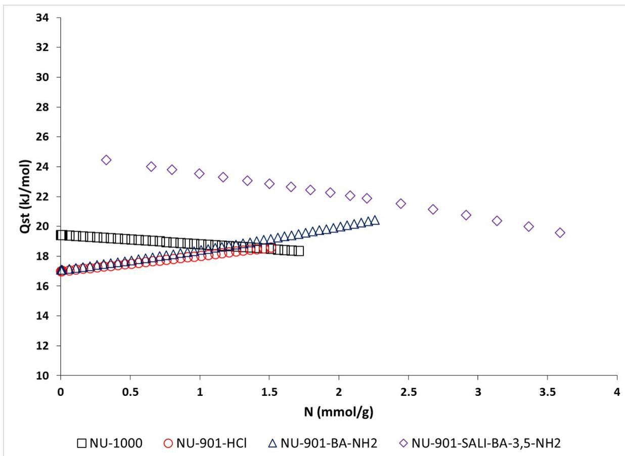
**Figure S18.** Plots of CO<sub>2</sub> isosteric heats of adsorption ( $Q_{st}$ ) of NU-1000 (black squares), NU-901-HCl (red circles), NU-901-BA-NH<sub>2</sub> (blue triangles), and NU-901-SALI-BA-3,5-NH<sub>2</sub> (purple diamonds) calculated from single-site Langmuir model from CO<sub>2</sub> isotherms recorded at 273, 283, and 293 K.
