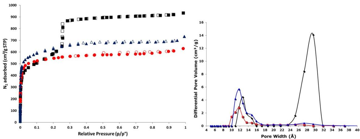
**Figure S11.** N<sub>2</sub> isotherms of NU-1000 (black squares), NU-901-BA-NH<sub>2</sub> (red circles), and NU-901-HCl (blue triangles). Adsorption = filled, desorption = empty markers.
