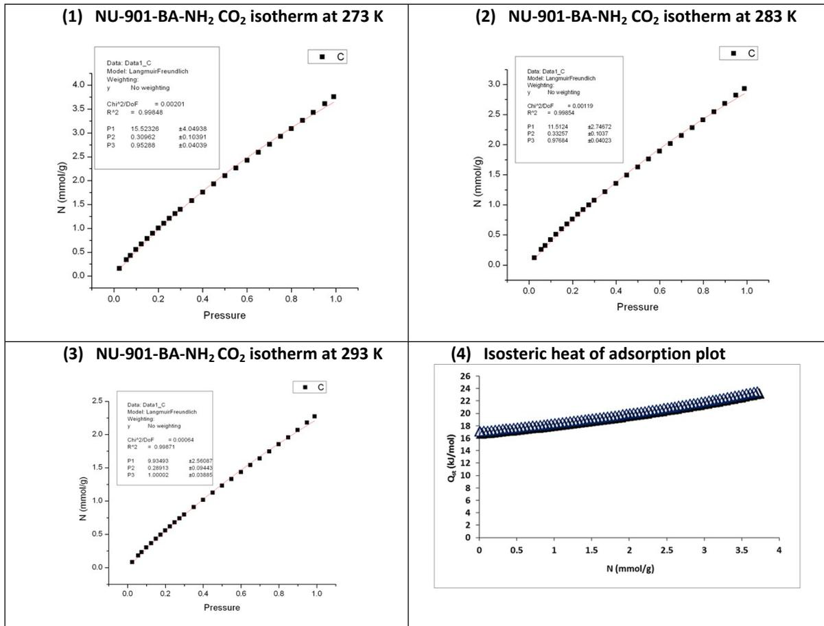
**Figure S20.** CO<sub>2</sub> adsorption curves, fitting and parameters for NU-901-BA-NH<sub>2</sub> at 273 K (1), 283 K (2), 293 K (3), and isosteric heat of adsorption ( $Q_{st}$ ) calculated by the single-site Langmuir-Freundlich model (4).
