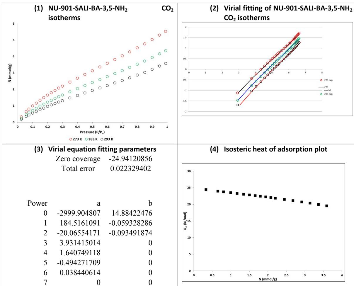
**Figure S22.** CO<sub>2</sub> adsorption curves (1), isotherm fitting (2), fitting parameters (3) and isosteric heat of adsorption ( $Q_{st}$ ) calculated by the Virial equation (4) for NU-901-SALI-BA-3,5-NH<sub>2</sub> at 273 K, 283 K, 293 K.
