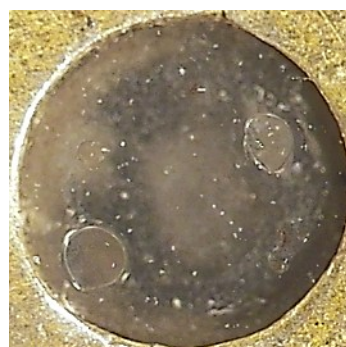
Image 8: At 161.0 °C all the crystals had fully melted.
