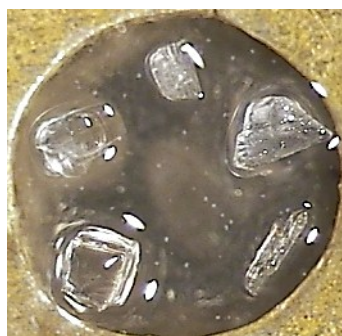
Image 4: At 132.1 °C the remaining polymorphs began to melt.
