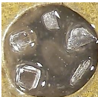
Image 2: At 122.8 °C the onset of opacity occurred within polymorph 3.
