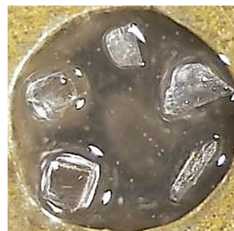
Image 3: At 128.9 °C the onset of the melt occurred for polymorph 6.
