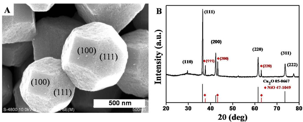
Figure S3. SEM image (A), XRD (B) of NiO/truncated octahedral Cu<sub>2</sub>O, proving NiO NCs were selectively grown on (111) facets of truncated octahedral Cu<sub>2</sub>O.
