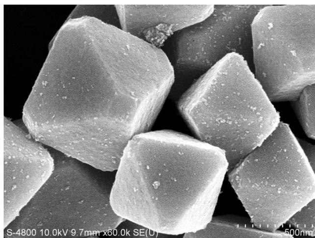
Figure S2. SEM image of Pd/truncated octahedral Cu<sub>2</sub>O prepared under no visible light irradiation, showing Pd NCs were preferentially grown on (111) facets.
