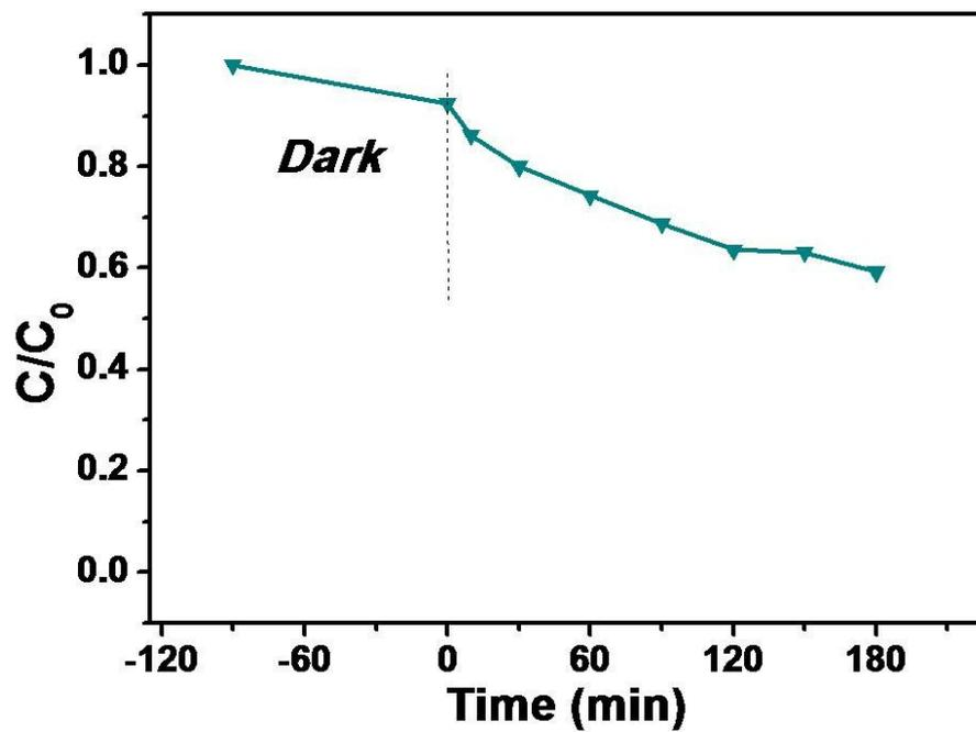
Figure S5. Photocatalytic activity at  $\lambda=254$  nm of Pd/(111)  $\text{Cu}_2\text{O}$  prepared under no light irradiation
