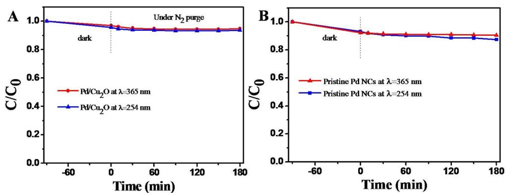
**Figure S6.** Two control experiments. (A) is, after using N<sub>2</sub> purge, photocatalytic activities of Pd/truncated octahedral Cu<sub>2</sub>O under single wavelength UV light irradiation. (B) is photocatalytic activities of pristine Pd NCs under single wavelength UV light irradiation.
