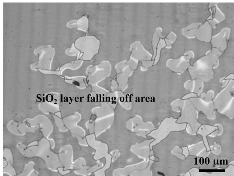
**Figure S3.** Optical microscope image of the -z surface of the PPMgLN sample after periodic poling, the thickness of the  $\text{SiO}_2$  dielectric layer is  $900\ \text{nm}$ .
