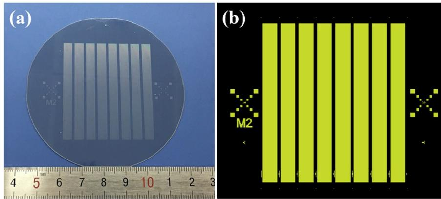
**Figure S4.** (a) Photograph of the product PPMgLN wafer. (b) Photomask designed for periodic poling.
