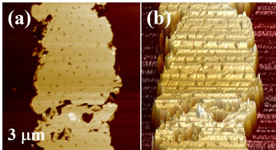
**Figure S5.** (a) Two-dimensional and (b) Three-dimensional AFM images of the inverted domains on the -z surface of the Mg:LN wafer after etching in hydrofluoric acid:
