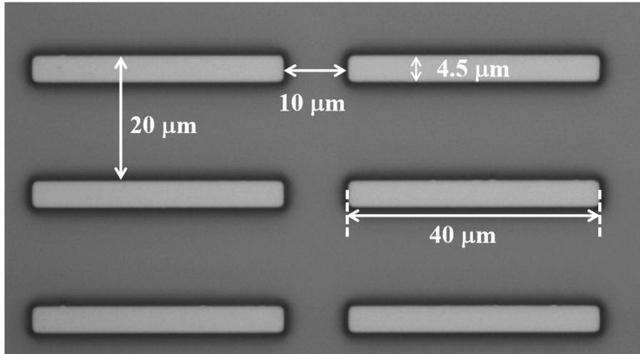
**Figure S2.** Optical microscope image of the patterned photoresist gratings on the +z surface of the Mg:LN wafer after hard bake.
