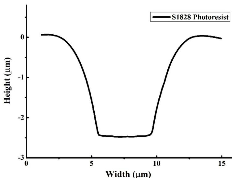
**Figure S1.** Typical profile of the trenches in the patterned photoresist after hard bake.
