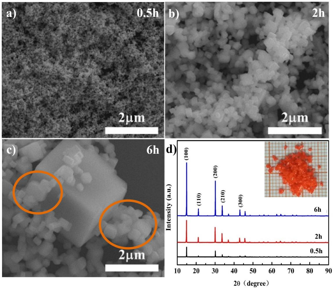
**Fig. S2.** SEM images of the MAPbBr<sub>3</sub> specimens prepared at different synthesis stages for (a) 0.5 h, (b) 2 h, and (c) 6 h. (d) All the XRD patterns are identical to those in Figure 1. The inset is the optical image of MAPbBr<sub>3</sub> powder prepared for 6h.
