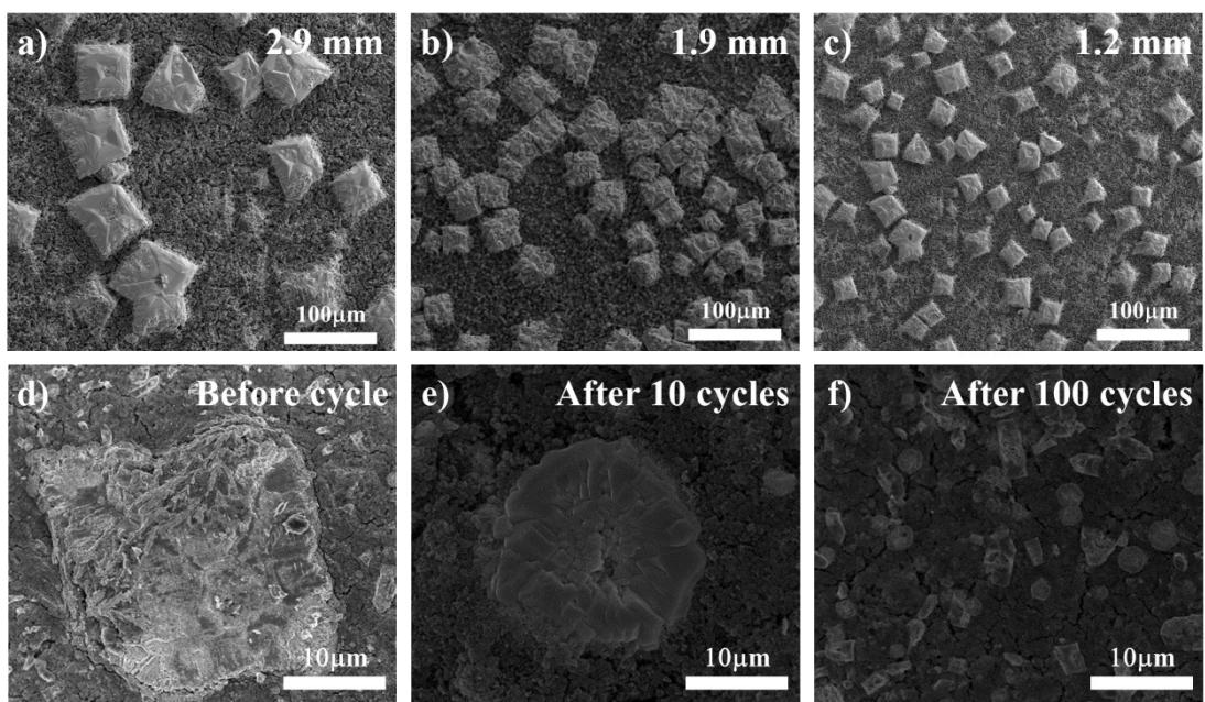
Fig.S3 SEM images of the as-prepared  $\text{CH}_3\text{NH}_3\text{PbBr}_3$  electrodes with different magnifications before and after different cycling test.
