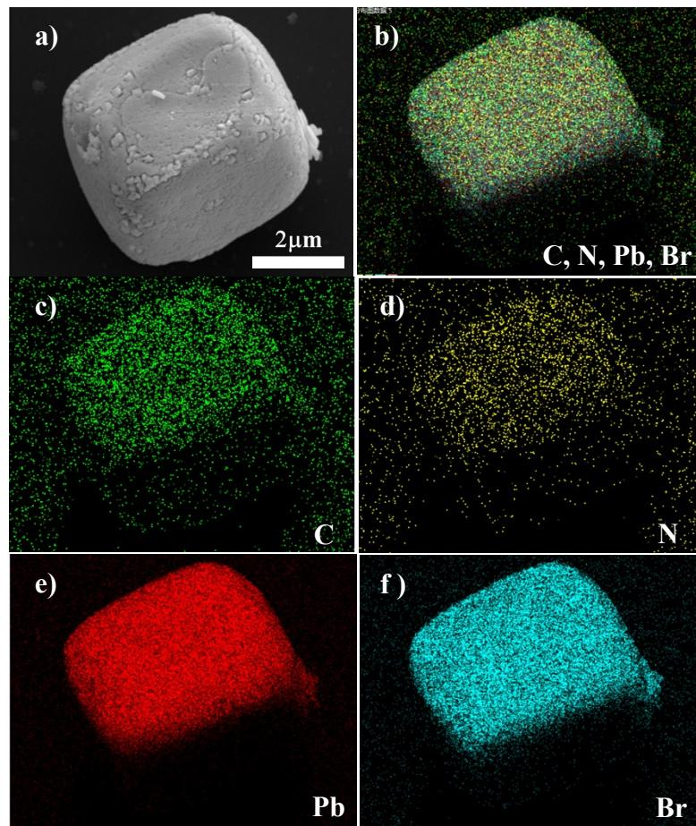
**Fig. S1.** SEM images (a) and (b-d) the EDS mapping spatially resolved C N, Pb and Te elemental mapping of the  $\text{MAPbBr}_3$  cubic microcrystal.
