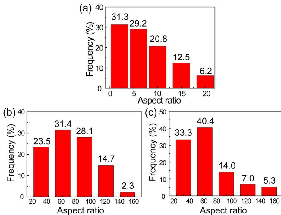
**Fig S2.** The aspect ratio distributions of the hydrothermal products prepared at 180 °C for 12.0 h with different initial OH<sup>-</sup> concentrations (mol L<sup>-1</sup>): (a) 0.287; (b) 0.575; (c) 2.300, while keeping the molar ratio of Ca<sup>2+</sup>:H<sub>3</sub>BO<sub>3</sub>:OH<sup>-</sup> as 1.000:4.625:14.375.
