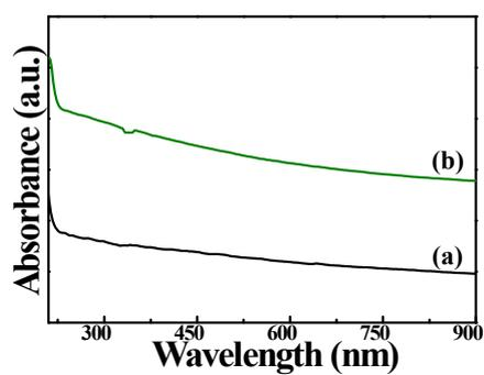
**Fig. S6.** UV-vis spectra of the  $\text{Ca}_2\text{B}_2\text{O}_5 \cdot \text{H}_2\text{O}:5.0\%\text{Eu}^{3+}$  (a) and  $\text{Ca}_2\text{B}_2\text{O}_5 \cdot \text{H}_2\text{O}:5.0\%\text{Tb}^{3+}$  (b) nanophosphors.
