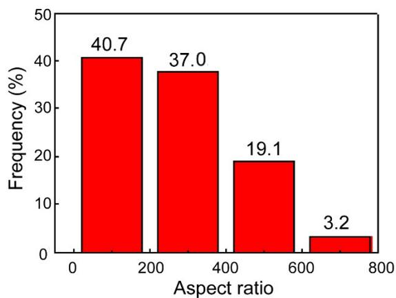
**Fig. S1.** Aspect ratio distribution of the  $\text{Ca}_2\text{B}_2\text{O}_5 \cdot \text{H}_2\text{O}$  nanowires hydrothermally synthesized at 180 °C for 12.0 h with molar ratio of  $\text{Ca}^{2+}:\text{H}_3\text{BO}_3:\text{OH}^-$  as 1.000:4.625:14.375.
