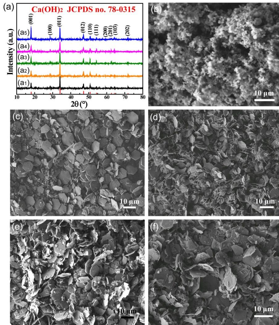
**Fig. S3.** XRD patterns (a) and SEM images (b-f) of the hydrothermal precursors obtained without (a<sub>1</sub>, b) and after treatment at various pre-treatment temperatures (a<sub>2</sub>- a<sub>5</sub>, c-f) for 30 min. Temperature (°C): (a<sub>2</sub>, c)-room temperature, (a<sub>3</sub>, d)-40, (a<sub>4</sub>, e)-60, (a<sub>5</sub>, f)-80. The red vertical lines in (a) indicate the standard pattern of Ca(OH)<sub>2</sub> (JCPDS no. 78-0315).
