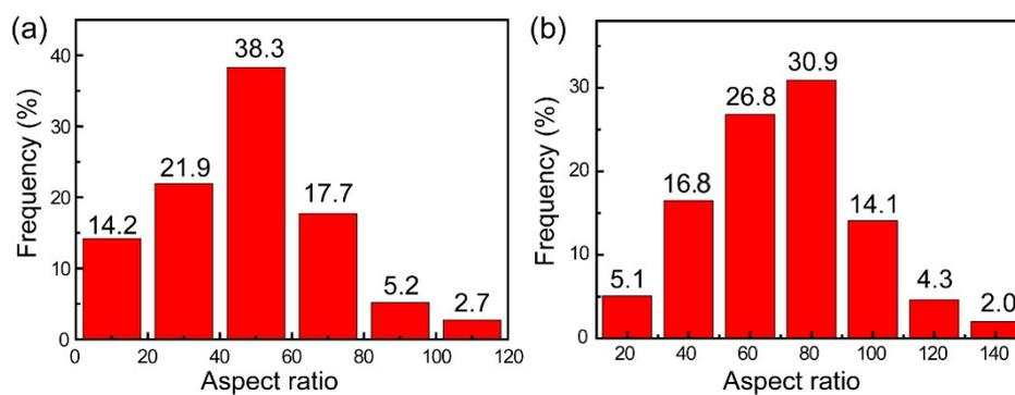
**Fig. S4.** Aspect ratio distribution of the hydrothermal products obtained at various temperatures for 12.0 h. Temperature (°C): (a)-120, (b)-150.
