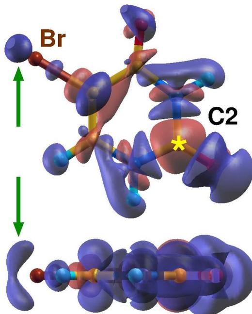
Figure 1 : Difference charge density map plotted with a 0.003 e/au<sup>2</sup> step of the isosurface sampling to better show the contribution of the Br atom to the screening of the C<sub>2</sub> 1s hole (top and side view)
