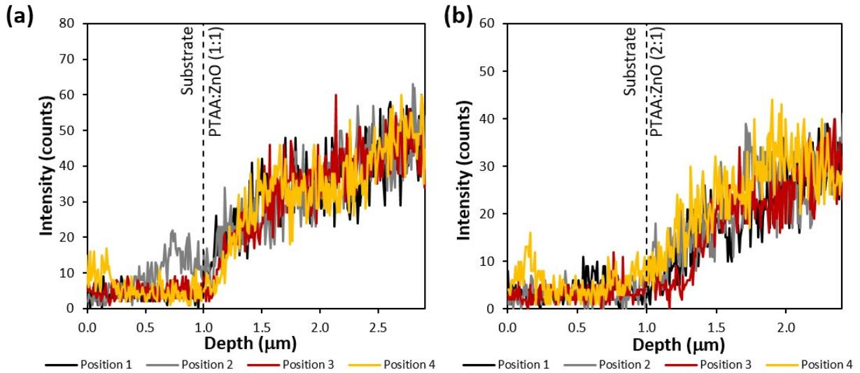
**Fig. S1.** The distribution of ZnO in the thick blended films corresponding to the active layers of (a) Device 1900-1:1 and (b) Device 1400-2:1, obtained via EDS. The four plotted curves were the result of vertical scans done in four positions across the films.
