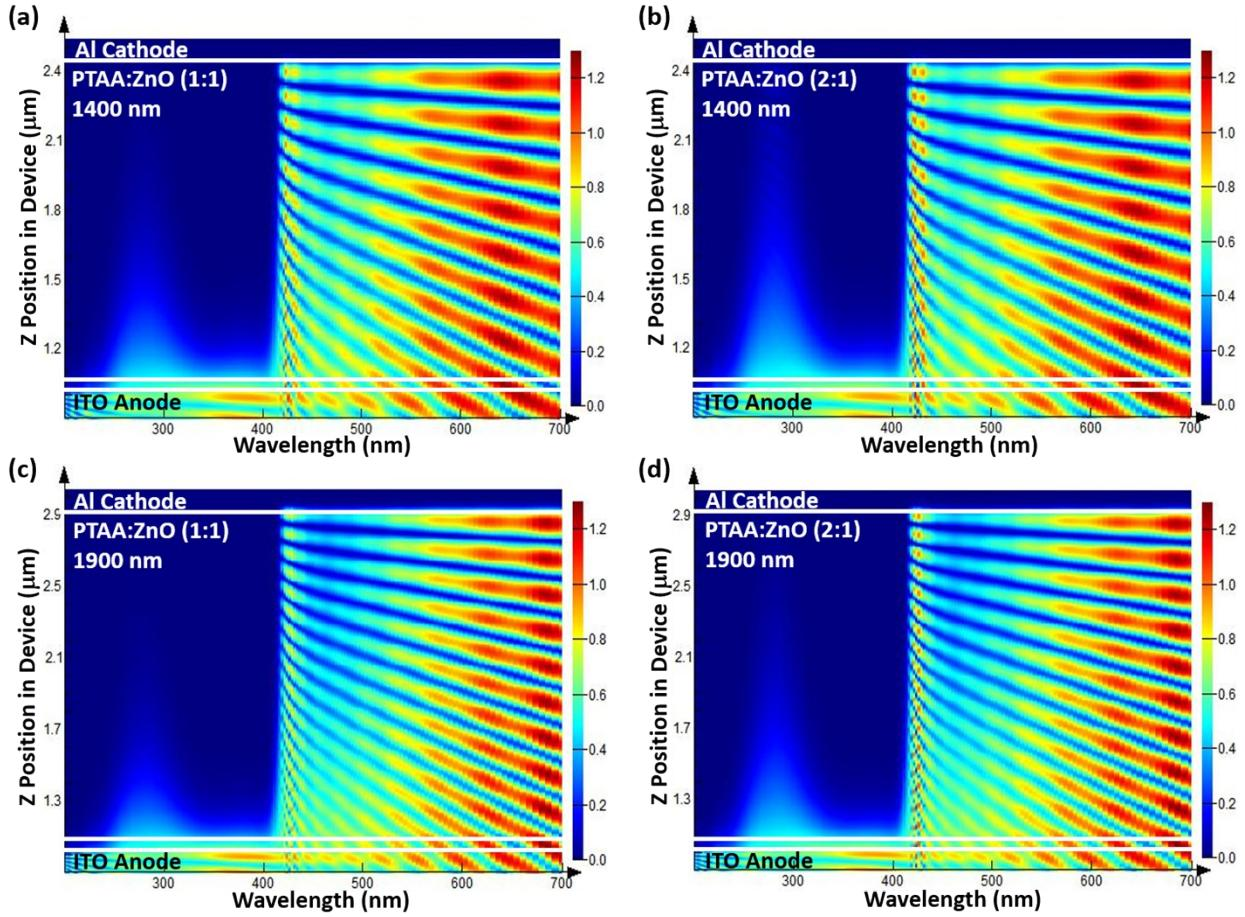
**Fig. S4.** Electric field distribution obtained via 3D-FDTD simulations for devices with (a) a PTAA:ZnO weight ratio of 1:1 and active layer thickness of 1400 nm, (b) a PTAA:ZnO weight ratio of 2:1 and active layer thickness of 1400 nm, (c) a PTAA:ZnO weight ratio of 1:1 and active layer thickness of 1900 nm, and (d) a PTAA:ZnO weight ratio of 2:1 and active layer thickness of 1900 nm.
