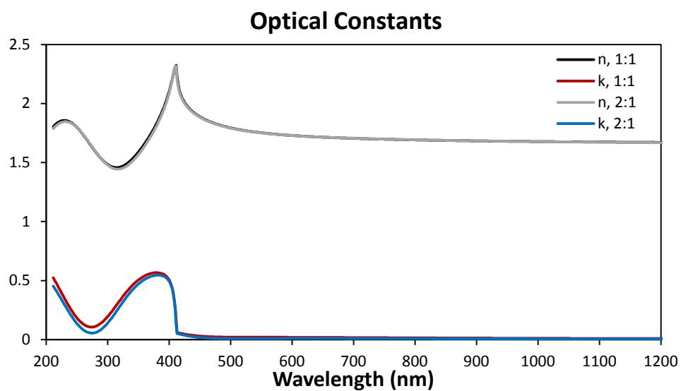
**Fig. S2.** The optical constants of refractive index,  $n$ , and extinction coefficient,  $k$ , for the blends of PTAA and ZnO with weight ratios of 1:1 and 2:1, as obtained via spectroscopic ellipsometry.
