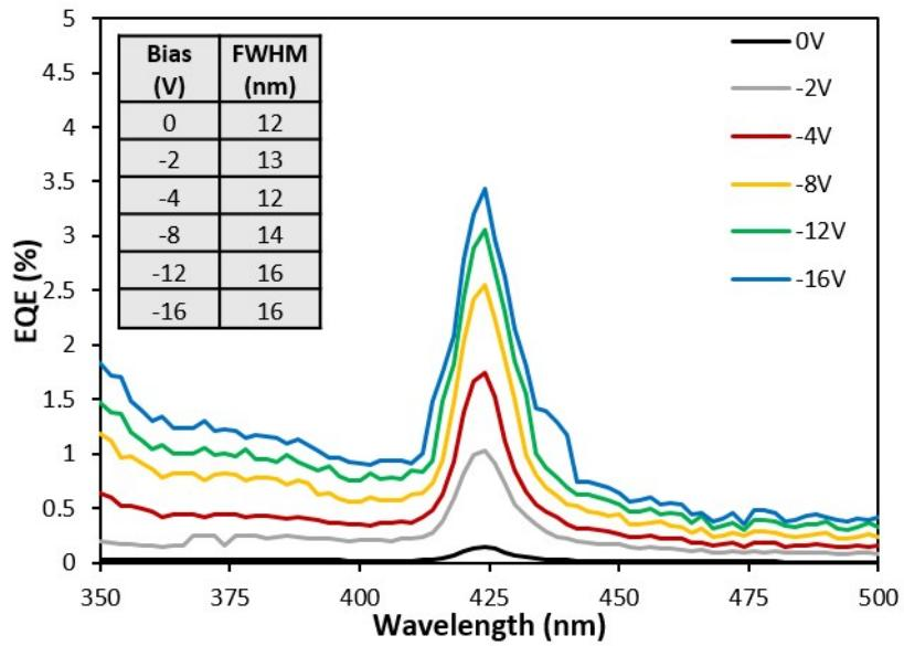
**Fig. S3.** EQE spectra for Device 1900-1:1 tested under strong reverse biases, demonstrating the stable shape of the curve and the stability of the FWHM values. Inset: Table of the FWHM values for each subsequent scan.
