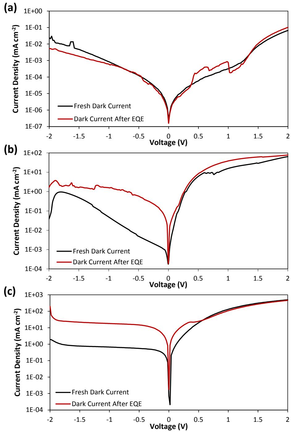
**Fig. S5.** Current density-voltage characteristics for (a) a pure PTAA device (ITO/PEDOT:PSS/PTAA/BCP/Al) with a 200 nm active layer, (b) a pure ZnO device (ITO/PEDOT:PSS/ZnO/BCP/Al) with a 260 nm active layer, and (c) a device with a PTAA:ZnO weight ratio of 1:10 and a 150 nm active layer.
