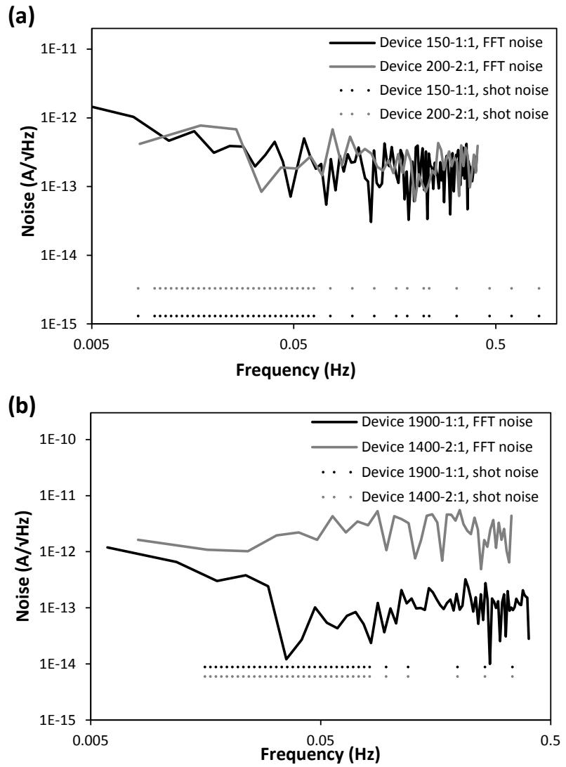
**Fig. S6.** Noise currents under no bias obtained from FFT and calculated shot noise approximations for (a) Devices 150-1:1 and 200-2:1, and (b) Devices 1900-1:1 and 1400-2:1.
