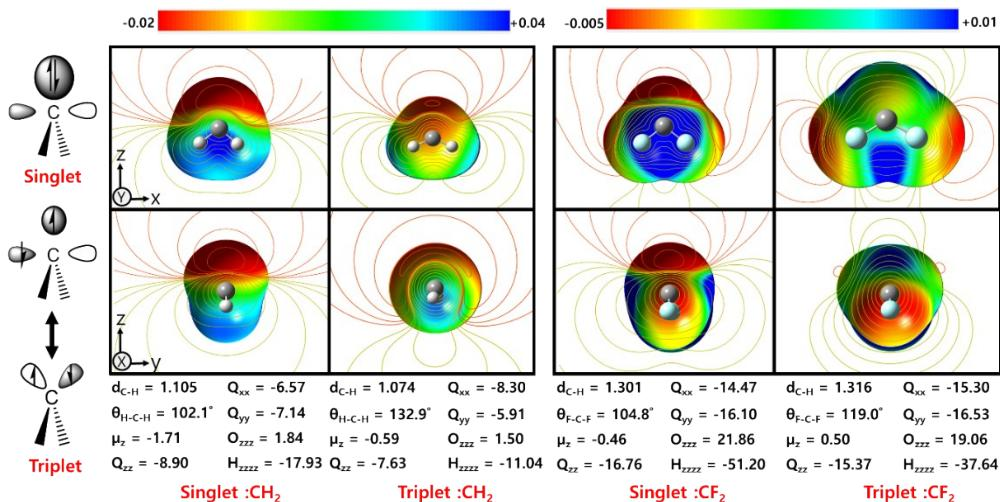
**Figure S1.** Electrostatic potential (EP) maps at the MP2/aVTZ of singlet/triplet states of CH<sub>2</sub> and CF<sub>2</sub>, with multipole moments at CCSD/aVTZ at the optimized CCSD(T)/aV5Z geometries (d: distance and  $\theta$ : angle). Distances are in Å; 2<sup>n</sup>-multipole moments [Dipole ( $\mu$ ), quadrupole ( $Q$ ), octupole ( $O$ ), and hexapole ( $H$ ) moments] in Debye·Å<sup>n-1</sup>.
