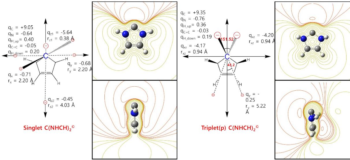
**Figure S4.** Multipole models for interaction potentials for imidazole-2-ylidene ( $\text{C}(\text{NHCH})_2^\circ$ ) which reproduce the EP maps of singlet and triplet-p  $\text{C}(\text{NHCH})_2^\circ$  at the CCSD/aVTZ//CCSD(T)/aVTZ level.
