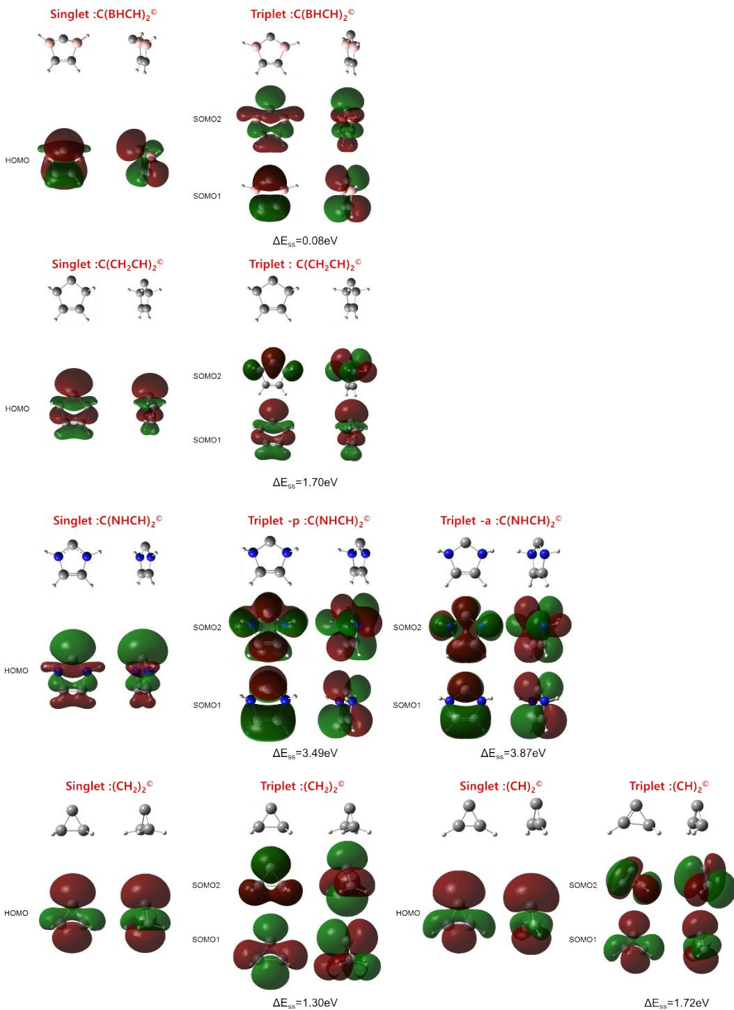
**Figure S14.** Frontier molecular orbitals of  $\text{C}(\text{BHCH})_2^{\circledcirc}$ ,  $\text{C}(\text{CH}_2\text{CH})_2^{\circledcirc}$ ,  $\text{C}(\text{NHCH})_2^{\circledcirc}$ ,  $(\text{CH}_2)_2^{\circledcirc}$  and  $:(\text{CH})_2^{\circledcirc}$  at the B3LYP/aVTZ level of theory.
