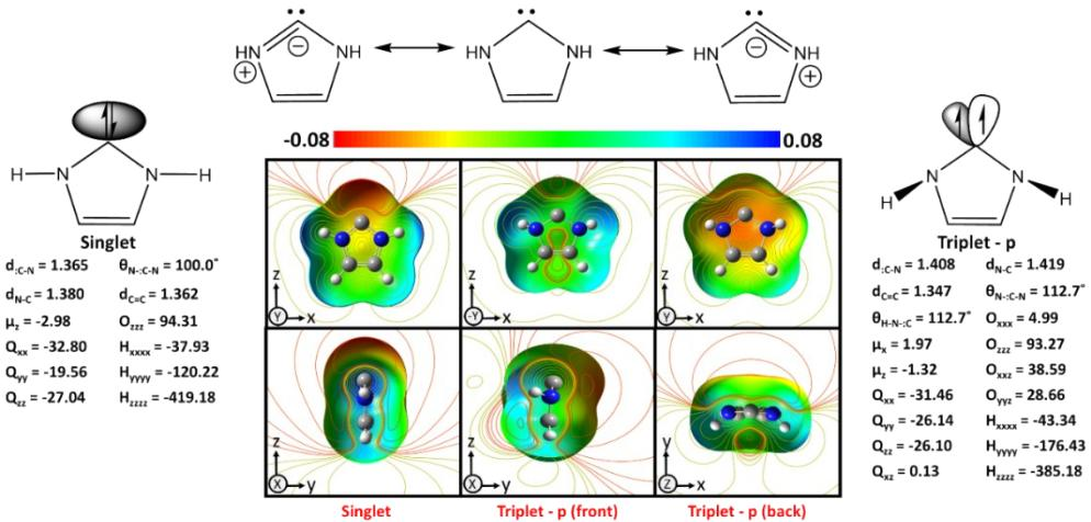
**Figure S2:** EP maps at the MP2/aVTZ level and multipole moments at the CCSD/aVTZ level on the optimized CCSD(T)/aVTZ geometries of singlet and triplet imidazol-2-ylidene ( $C(NHCH)_2^\circ$ ). Distances are in Å;  $2^n$ -multipole moments in Debye·Å $^{n-1}$ .
