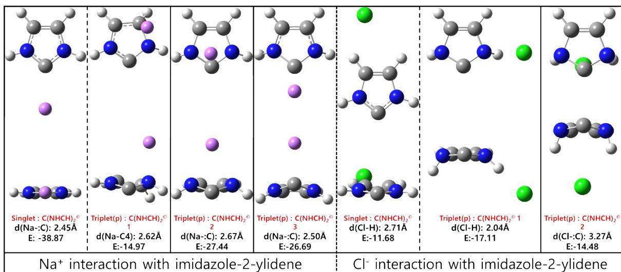
**Figure S7.** Interactions of singlet and triplet-p(parallel)  $C(NHCH)_2^\circ$  with a  $Na^+/Cl^-$  ion and  $H_2O$ . E (kcal/mol) is the interaction energy at the CCSD(T)/CBS level on the MP2/aVTZ geometry. d is interatomic distance.
