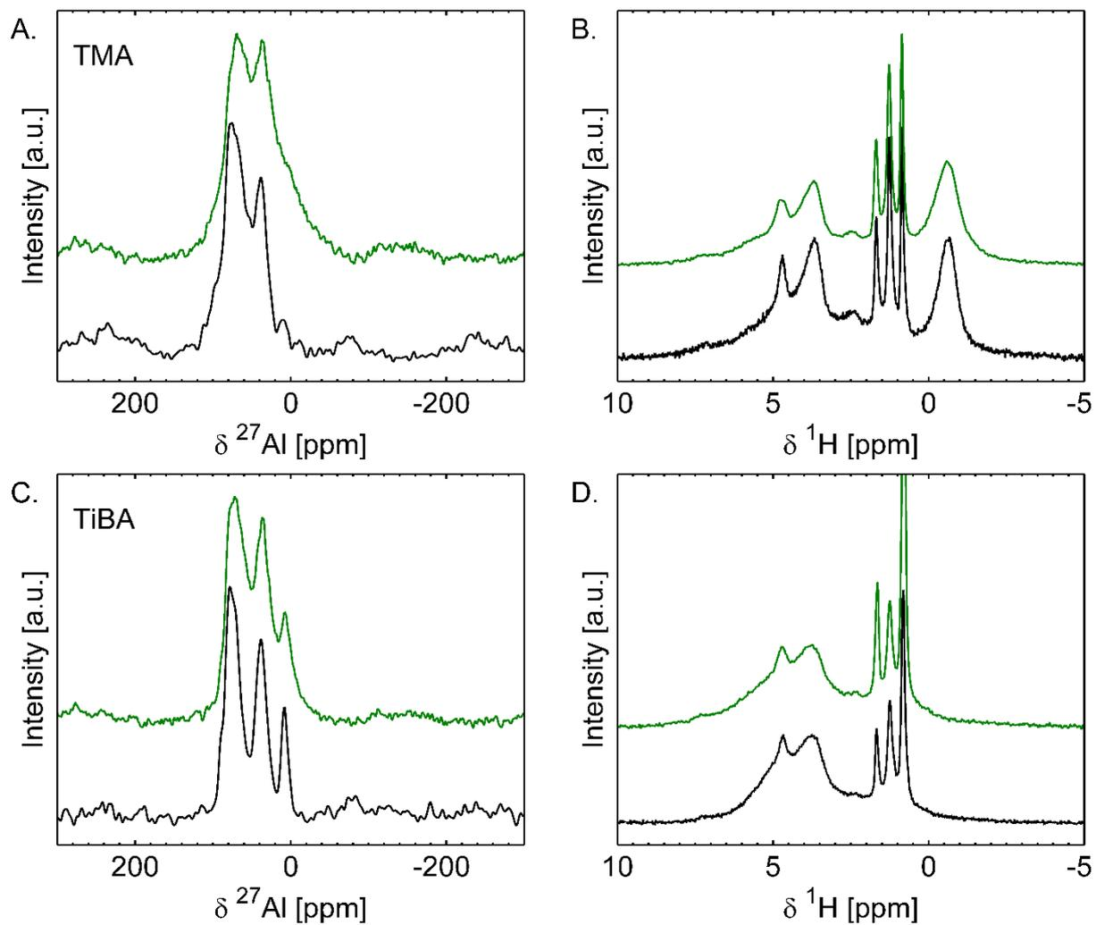
Figure SI 3: (A., C.)  $^{27}\text{Al}$  and (B., D.)  $^1\text{H}$  MAS NMR spectra of MC-M (A., B.) and MC-B (C., D.) adducts at fields of 14.1 T (green) and 20 T (black); MAS speed = 30 and 35 kHz, respectively.
