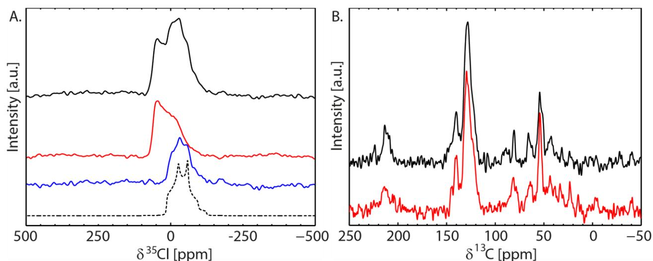
Figure SI 10: A.  $^{35}\text{Cl}$  MAS and B.  $^{13}\text{C}$  CP MAS spectra for Do2-MD at 20.0 T measured before exposure (red) and after a long exposure of the sample (black). The 'before' signal in the  $^{35}\text{Cl}$  spectrum is displayed at 28 % of its original intensity, the blue line shows the difference between the black and red curve and the dotted line is a simulation.
