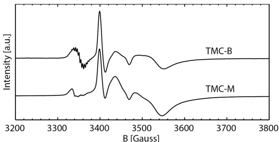
Figure SI 7: Room temperature X-band EPR spectrum for TMC-B (top) and TMC-M (bottom).
