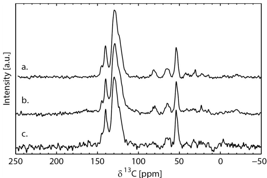
Figure SI 8:  $^{13}\text{C}$  MAS spectra for a. binary, b. ternary and c. quaternary system containing the DMFluo donor at 9.4 T using 75 kHz  $^1\text{H}$  decoupling and MAS speeds of 15-18 kHz.
