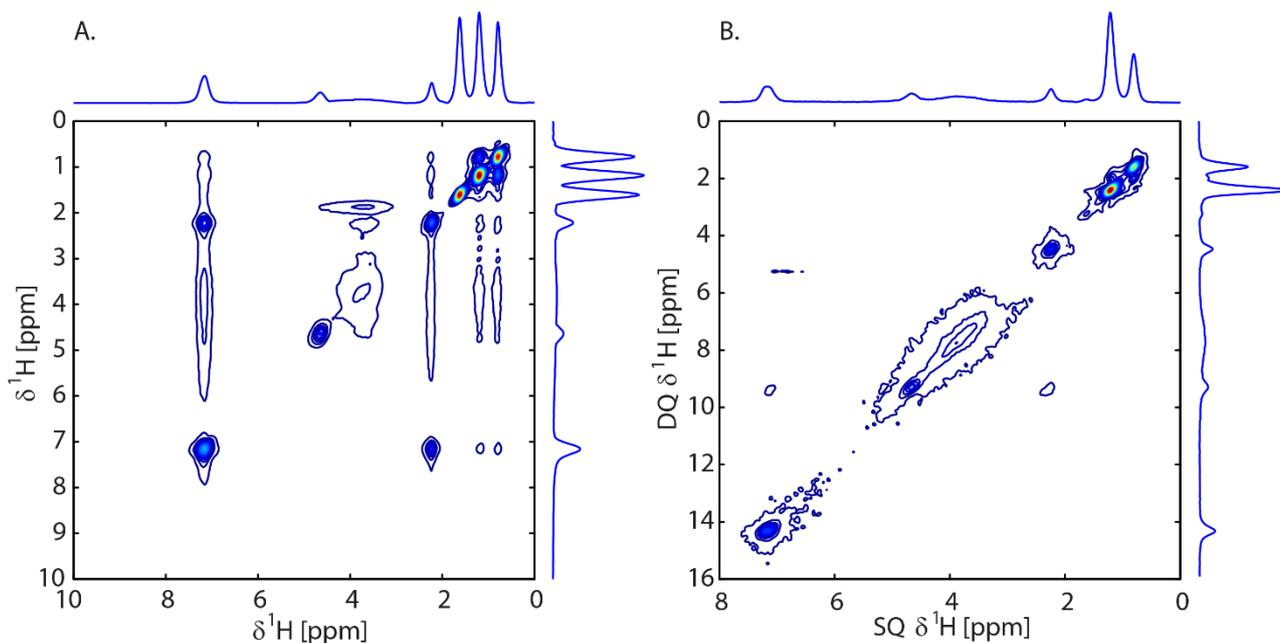
Figure SI 4: 2D correlation spectra for MC-M, showing A.  $^1\text{H}$  2D Exchange spectrum at an exchange time of 100 ms and B.  $^1\text{H}$  2D DQSQ spectrum.
