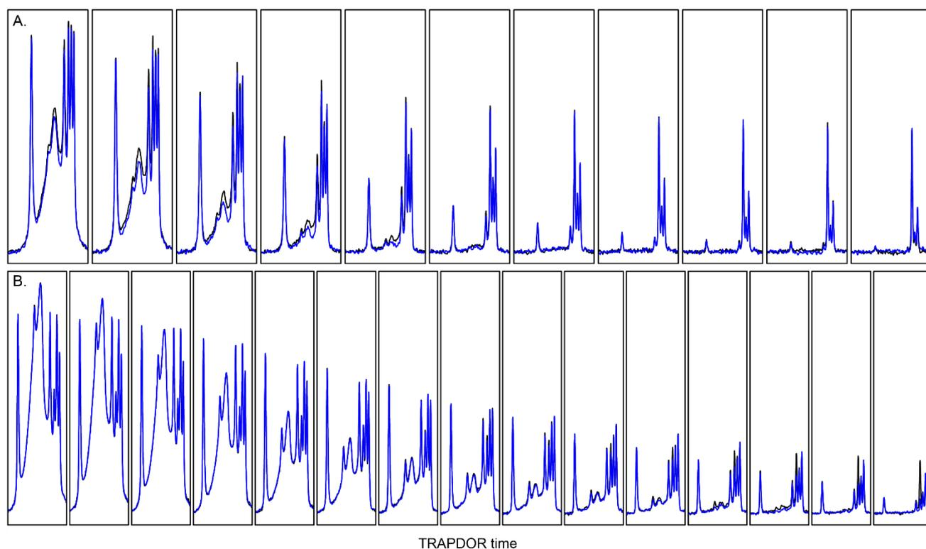
Figure SI 5:  $^1\text{H}\{-^{27}\text{Al}\}$  and B.  $^1\text{H}\{-^{35}\text{Cl}\}$  TRAPDOR experiment for the degraded MC-M at  $B_0 = 20.0$  T. Total TRAPDOR dephasing time is 16 ms in A. and 17 ms in B., while the MAS speed is 12.5 and 35 kHz respectively,  $v_{\text{RF}}^{27\text{Al}} = 120$  kHz and  $v_{\text{RF}}^{35\text{Cl}} = 30$  kHz.
