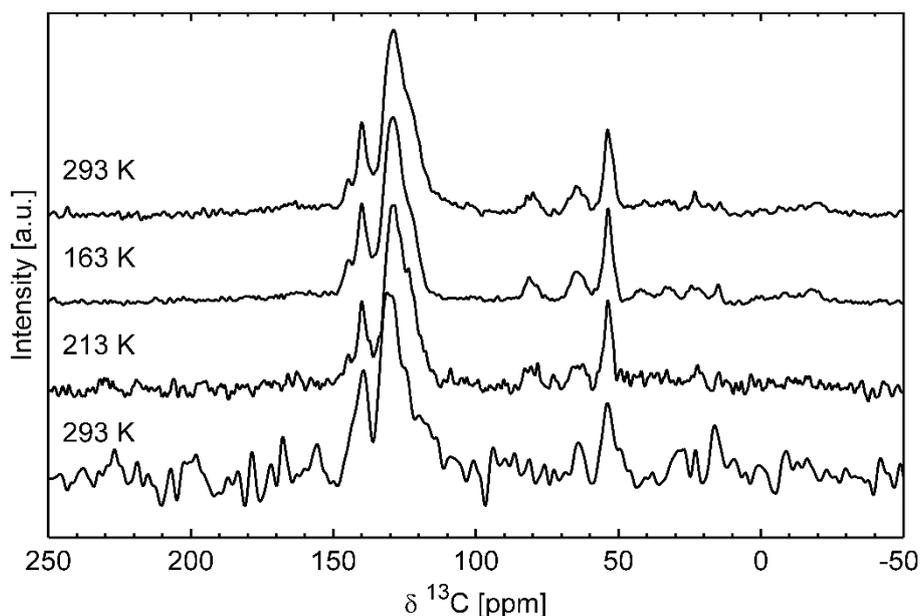
Figure SI 9:  $^{13}\text{C}$  MAS spectrum of Do2-M at various temperatures at 9.4 T showing the spectra before (bottom) and after (top) a cooling cycle. The bottom spectrum was acquired using 50 kHz  $^1\text{H}$  decoupling, while 75 kHz  $^1\text{H}$  decoupling was used for the other spectra.
