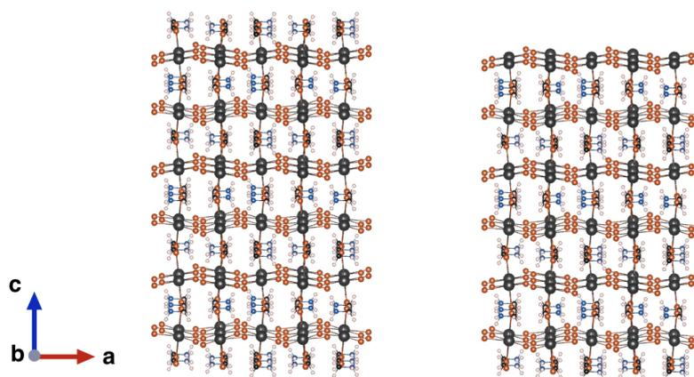
**Fig. S1** (001) slabs terminated with MA-Br (left) and Pb-Br (right). The most stable surface is found to be the MA-Br terminated one [Komesu *et al.*, *J. Phys. Chem. C* **2016**, *120*, 21710].
