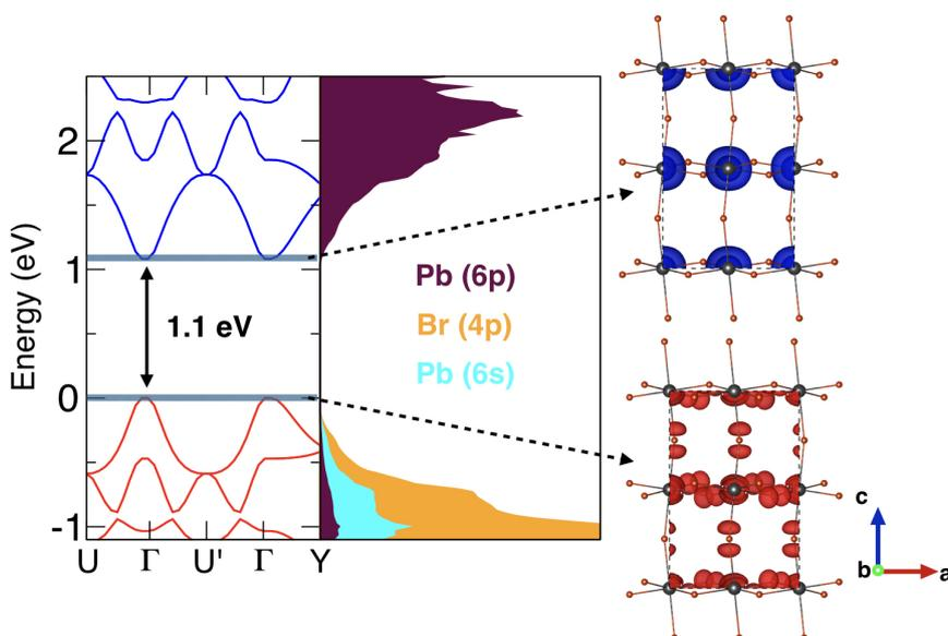
**Fig. S2** Electronic properties of bulk MAPbBr<sub>3</sub>. (left panel) Electronic dispersion evidencing a direct band gap (1.1 eV) at the center of the Brillouin Zone ( $\Gamma$ ) computed with SOC. (middle panel) Projected densities of states. (right panel) LDOS illustrating the major contribution of Br(4p) and Pb(6s) in VBM and Pb(6p) in CBM.
