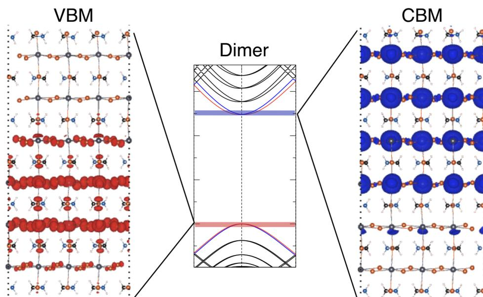
**Fig. S3** LDOS of VBM and CBM of the relaxed slab in its dimer configuration, to be compared to those obtained for the zigzag configuration reported in Figure 4c, revealing similar features.
