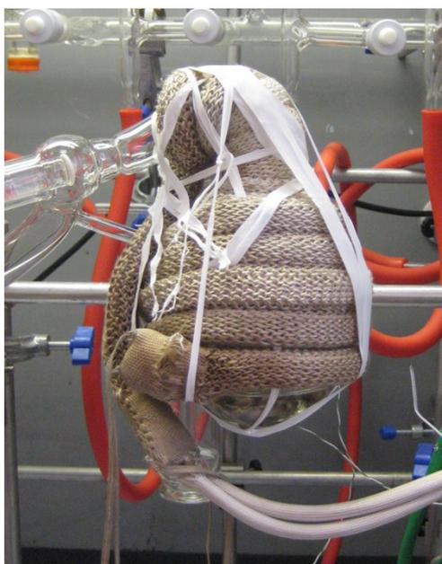
**Figure S1** The heating tape around the distillation pot, supported with PTFE tape. The base was left uncovered and the entire pot was subsequently covered in several layers of glass wool.
