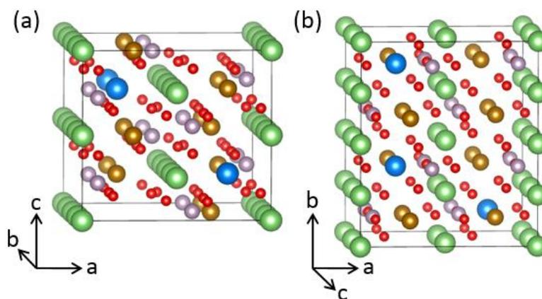
**Fig. S2** Schematic for the structure of  $\text{Li}_{1+x}\text{Fe}_{1-x}\text{PO}_4$  ( $x = 18.75\%$ ). (a) in  $ac$  plane; (b) in  $ab$  plane.
