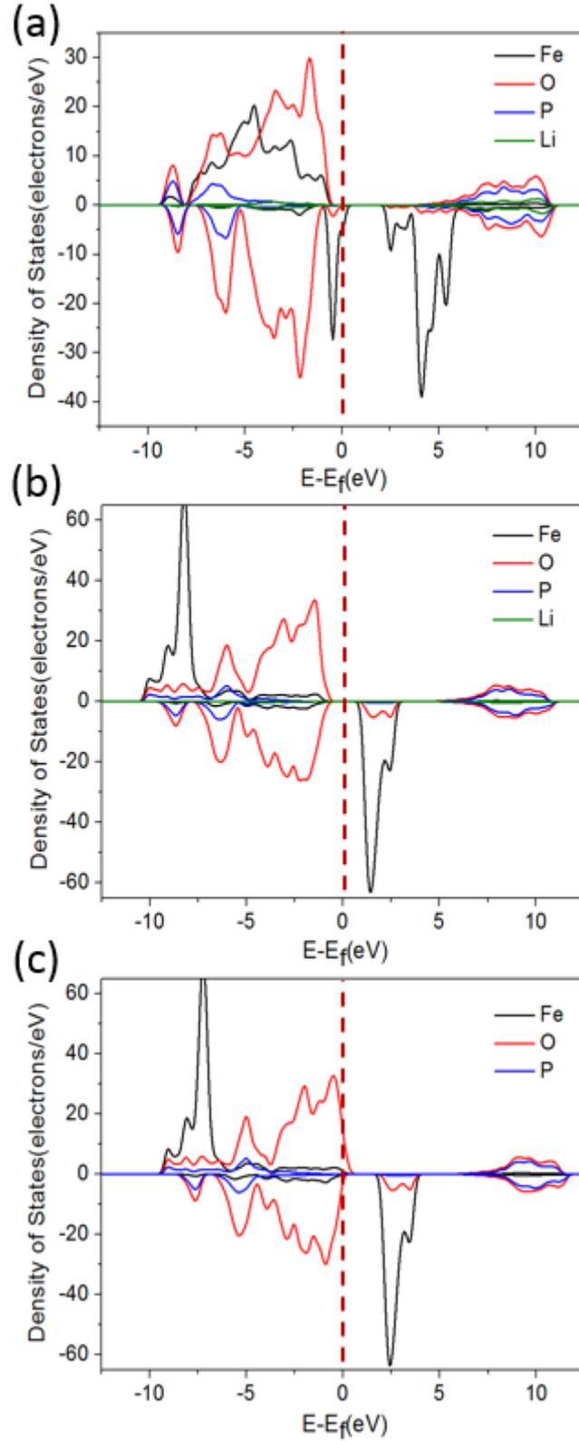
**Fig. S5** The PDOS of  $\text{Li}_{1+x-y}\text{Fe}_{1-x}\text{PO}_4$  ( $x = 6.25\%$ ). (a)  $y = 0$ ; (b)  $y = 1-2x$ ; (c)  $y = 1+x$ .
