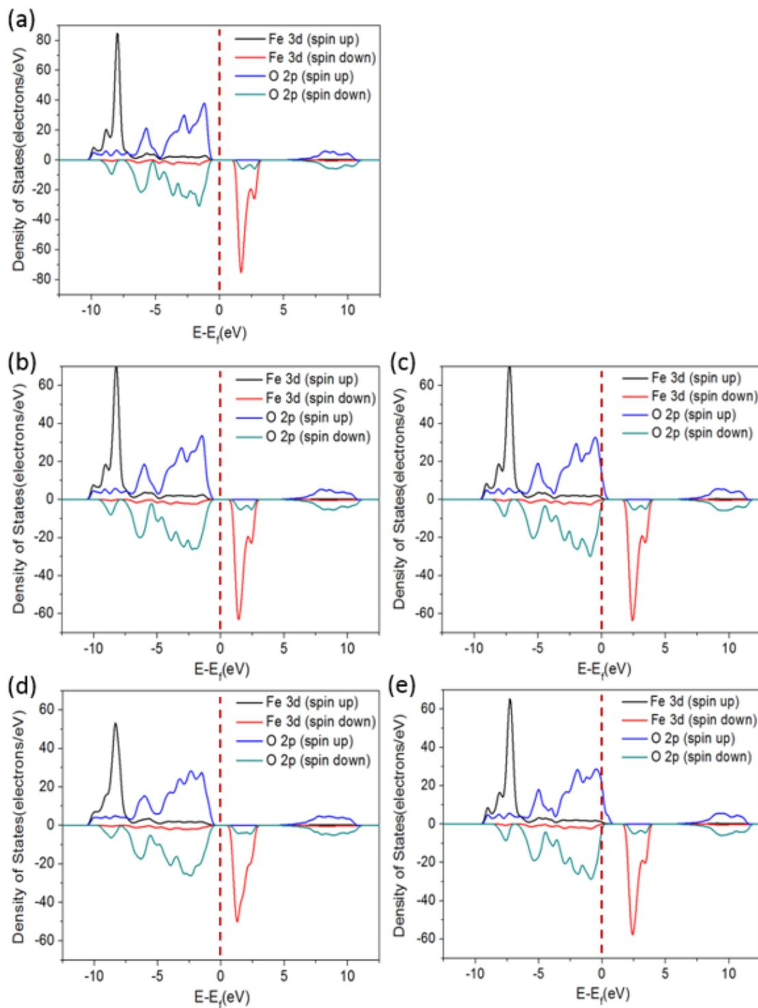
**Fig. S4** The PDOS of  $\text{Li}_{1+x-y}\text{Fe}_{1-x}\text{PO}_4$ . (a)  $x = 0, y = 1+x$ ; (b)  $x = 6.25\%, y = 1-2x$ ; (c)  $x = 6.25\%, y = 1+x$ ; (d)  $x = 12.5\%, y = 1-2x$ ; (e)  $x = 12.5\%, y = 1+x$ . The Fermi level (the vertical red dashed line) is set to zero energy.
