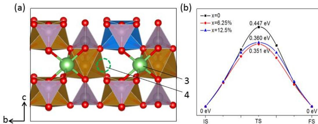
**Fig. S6** (a) Schematic for the structure of  $\text{Li}_{1+x}\text{Fe}_{1-x}\text{PO}_4$ . 3 stands for a Li-ion, and 4 stands for a Li-vacancy in the  $[010]$  channel. (b) The energy barriers for a Li-ion to hop from the 3 site to the 4 site in the bulk  $\text{Li}_{1+x}\text{Fe}_{1-x}\text{PO}_4$  ( $x = 0, 6.25\%$  and  $12.5\%$ ).
