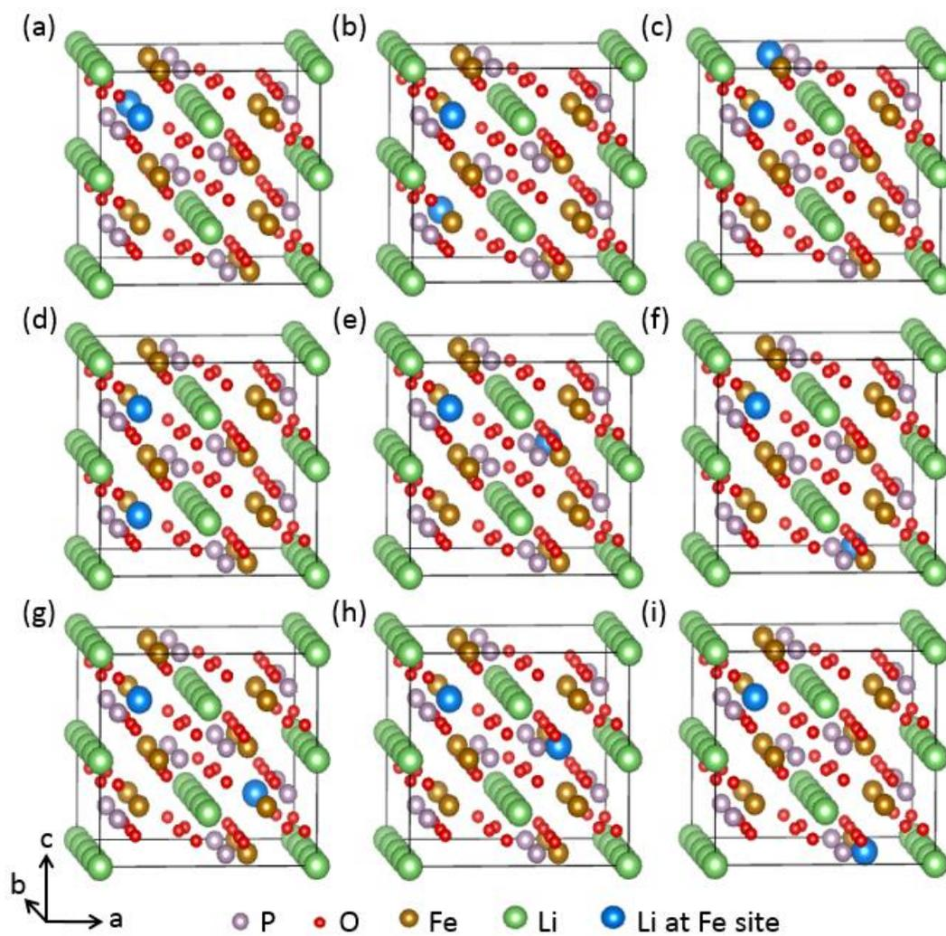
**Fig. S1** (a-i) Schematics for different structures of  $\text{Li}_{1+x}\text{Fe}_{1-x}\text{PO}_4$  ( $x = 12.5\%$ ). The total energies of them are -759.036, -758.512, -758.964, -758.441, -758.399, -758.384, -758.961, -758.894 and -758.284 eV, respectively.
