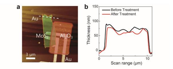
**Figure S1:** (a) The atomic force microscopy (AFM) image and (b) AFM height profile along the white line in the AFM image before (black line) and after (red line) hydrogen treatment. The average thickness of exfoliated few-layer  $MoS_2$  after the treatment is reduced by 9.85 nm after the treatment.
