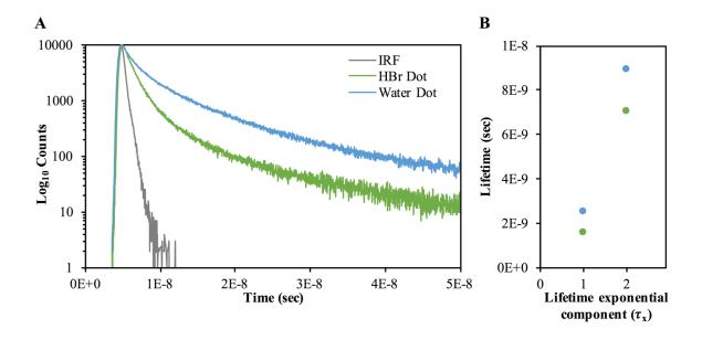
**Figure S4.** Fluorescence intensity decays ( $\lambda_{ex,em} = 311/350 \text{ nm}$ ) of carbon nanodots collected into water versus heavy carbon nanodots collected into 5M HBr over a 4 hour burn time. Samples were taken into glycerol and then analyzed at an equivalent pH. **A** – Intensity decays analyzed by TCSPC method. **B** – Plot of reported lifetime versus exponential component of decay model.
