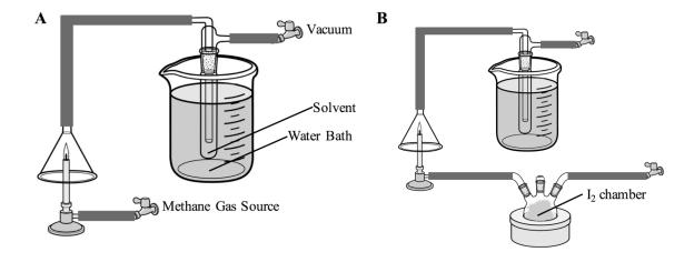
**Scheme S1.** Experimental production of carbon nanodots. **A** – Standard collection method. **B** – Altered production method for collection of iodated nanodots.
