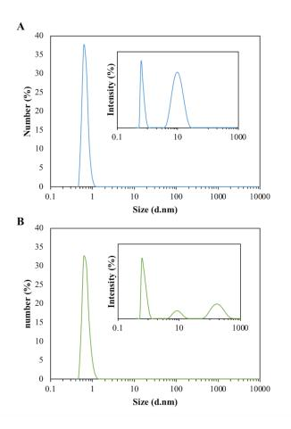
**Figure S3.** Diameter of carbon nanodot structures as analyzed by dynamic light scattering techniques. A - Size distribution by number of carbon nanodots collected into water. The inset is distribution by intensity. B - Size distribution by number of brominated carbon nanodots. The inset is distribution by intensity.
