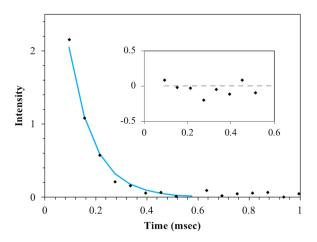
**Figure S2.** Phosphorescence intensity decay of brominated carbon nanodots (4hr) with single exponential fit. Inset represents the fit residuals. Collection parameters:  $\lambda_{ex} = 300$ nm,  $\lambda_{em} = 550$  nm, Gate time = 0.05 msec, Delay time = 0.07 msec.
