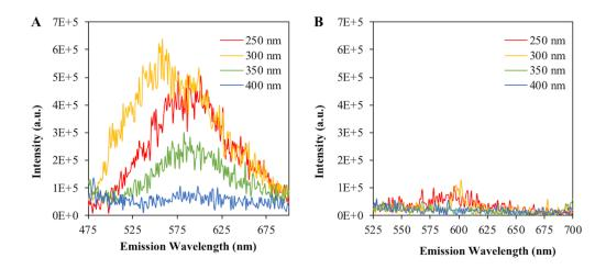
**Figure S5.** Phosphorescence emission spectra for heavy carbon nanodots collected into 5M HBr versus that of carbon nanodots collected into water. Both samples were taken into glycerol and analyzed at at equivalent pH values for excitation wavelengths including 250, 300, 350, and 400 nm. **A** – Emission spectra versus wavelength for heavy carbon nanodots. **B** – Phosphorescence emission spectra for carbon nanodots collected into water over the same excitation range.
