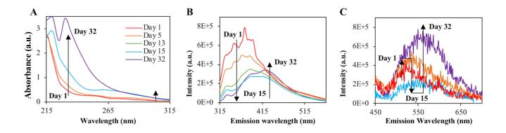
**Figure S7.** Luminescence stability of heavy carbon nanodots collected into 5M HBr for 4 hours. The sample was prepared as a glycerol mixture and kept stirring just above room temperature for the period of 1 month. The sample was periodically removed, analyzed, and returned to the mixing conditions. **A** – Sample absorbance. **B** – Sample fluorescence, excited at 300 nm. **C** – Sample phosphorescence, excited at 300 nm.
