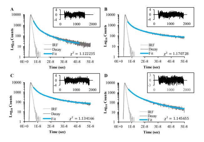
**Figure S8.** Analysis of fluorescence intensity decays of brominated carbon nanodots collected into 5M HBr over 4 hours. Samples were pH adjusted, diluted to equal concentrations, then analyzed in glycerol. Insets indicate residual values for each model fit. ( $\lambda_{ex} = 311 \ nm$ ,  $\lambda_{em} > 350 \ nm$ ) **A** – Sample as collected, pH = 0.22. **B** – Basic sample, pH = 13.61. **C** – Acidic sample, pH = 1.28. **D** – Neutral sample, pH = 7.33.
