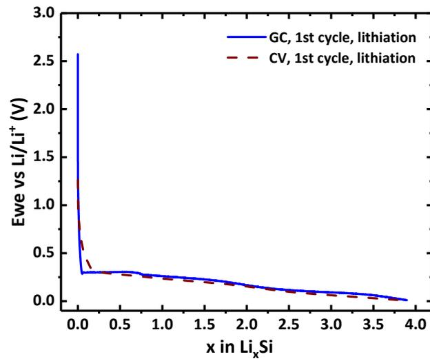
**Fig. S5:** Electrode potential  $E_{we}$  as a function of Li fraction  $x$  in  $\text{Li}_x\text{Si}$  during lithiation as calculated from electrochemical measurements (first cycle) according to eq. (S1) for the CV measurements shown in S4 and for galvanostatic charging of a different but similar silicon electrode with  $40 \mu\text{A}$  (GC).
