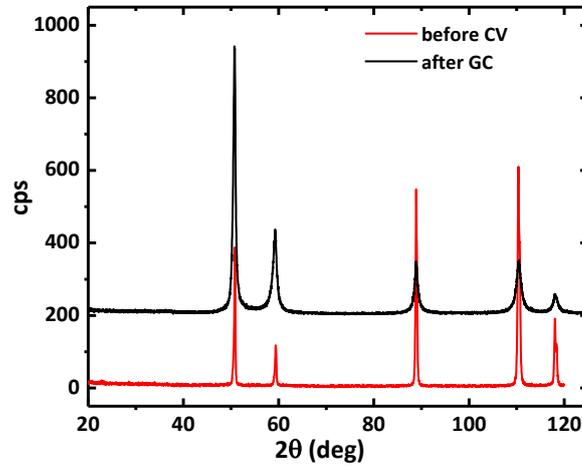
**Fig. S1:** Grazing incidence X-ray diffraction pattern of the silicon electrode before CV measurements were done (before CV). Only intense sharp Bragg peaks from the copper current collector are visible. Also shown is the pattern of an electrode with a similar silicon thickness of 400 Å after galvanostatic cycling at different charging rates (after GC). No additional peaks are observed. The patterns are shifted for clarity.
