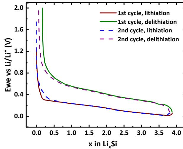
**Fig. S4:** Electrode potential  $E_{\text{we}}$  as a function of Li fraction  $x$  in  $a\text{-Li}_x\text{Si}$  for the two cycles of the CV measurements ( $x$  calculated from CV measurements according to eq. (S1)).
