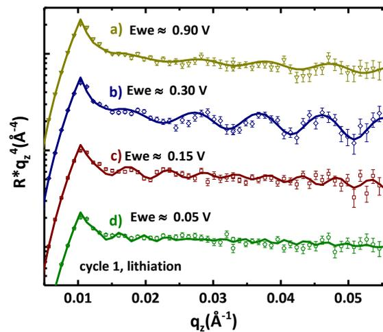
**Fig. S2:** Neutron reflectivity (R) patterns from Fig. 2(a) of the main manuscript plotted as  $R \cdot q_z^4$  vs.  $q_z$ .
