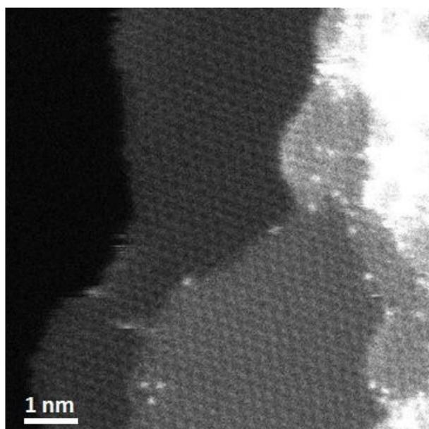
Fig. S1 Graphene sheet without nanopores prepared by arc-discharge in water.
