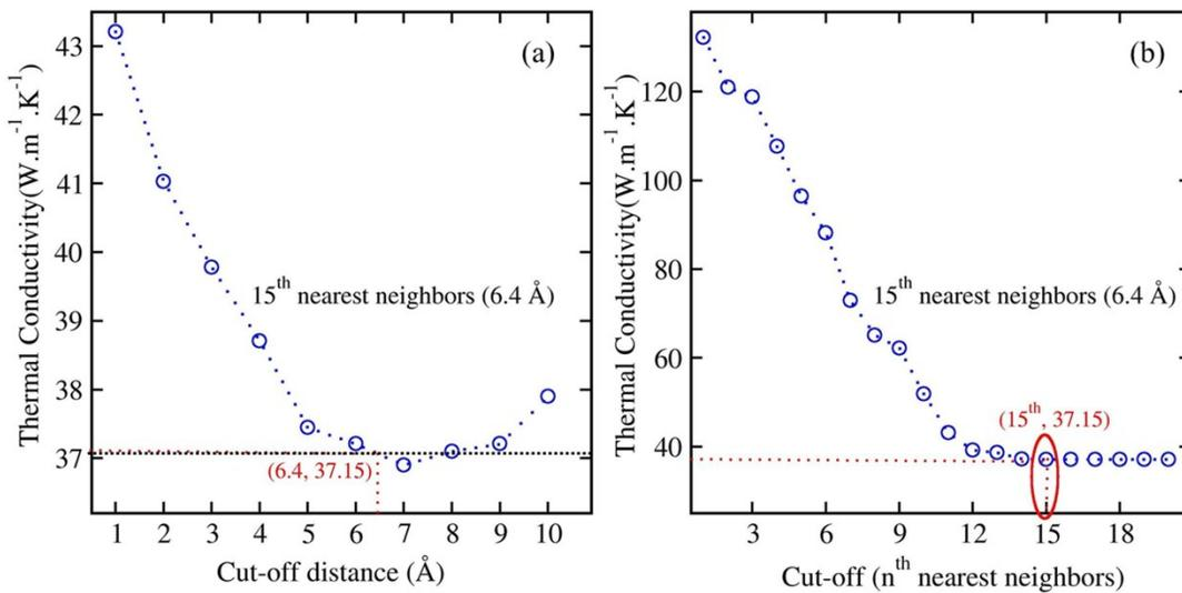
**Fig. S1:** Variation in thermal conductivity value with respect to (a) cut-off interaction distance in Å and (b) nearest neighbors for MLBP with the cubic force constant at 300 K. The red color ellipse shows the convergence of thermal conductivity at 15<sup>th</sup> nearest neighbors within 5 % with a cut-off radius of 6.4 Å by solving the linearized phonon BTE.
