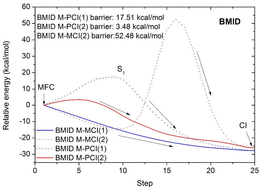
**Fig. S3** OM2/MRCI energy profiles along four paths for azoheteroarene BMID, generated by linear interpolation between the Franck-Condon geometry of the M-helical Z-isomer (MFC) and four different S<sub>1</sub>/S<sub>0</sub> conical intersections shown in Figure 3 in the main text of the article (MCI(1), PCI(1), MCI(2) and PCI(2)). Energies of BMID are relative to the S<sub>1</sub> excited-state energy of Franck-Condon geometry of its M-helical Z-isomer.
