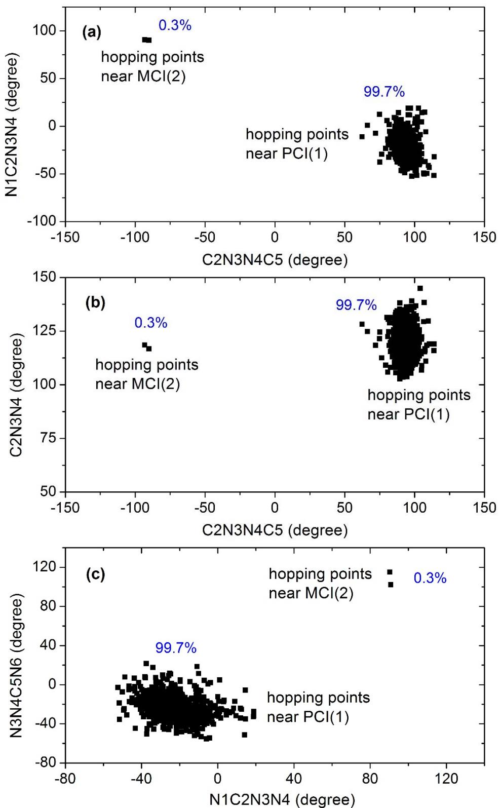
**Fig. S4** Distributions of the (a) C2N3N4C5 and N1C2N3N4 dihedral angles; (b) C2N3N4C5 dihedral angle and C2N3N4 bond angle; (c) N1C2N3N4 and N3N4C5N6 dihedral angles at the hopping points of 694 trajectories starting from *P*-helical Z-isomer of azoheteroarene BMID.
