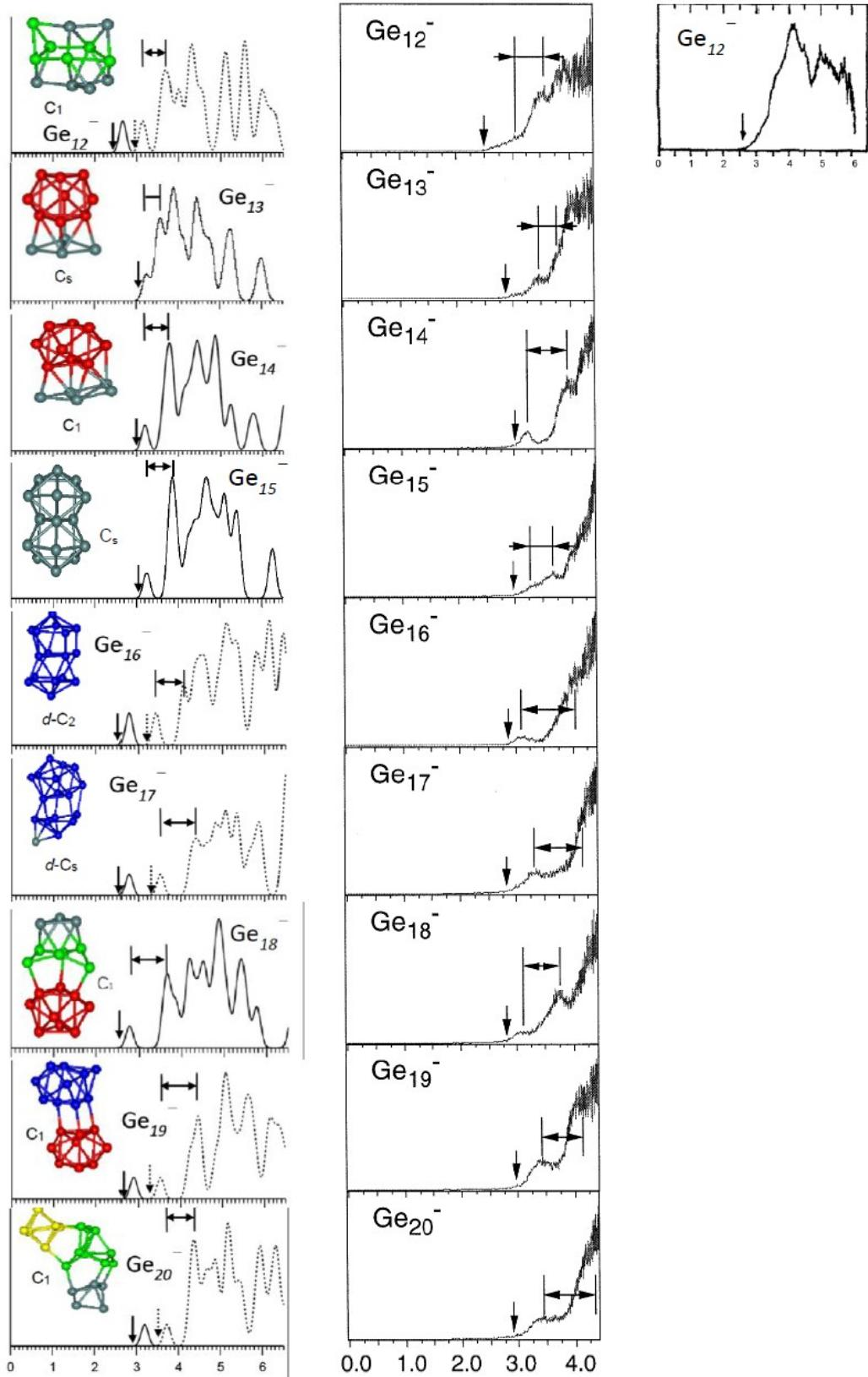
**Figure S2.** Simulated anion photoelectron spectra for the most likely isomers **a** of  $\text{Ge}_n^-$  ( $3 \leq n \leq 20$ ) displayed side-by-side with experimental spectra retrieved from the literatures (a: ref.<sup>1</sup>; b: ref.<sup>2</sup>).
