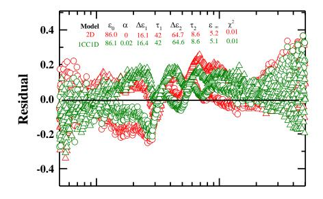
**Fig. S2:** A representative comparison between the two fitting models. Circles and triangles represent the real and imaginary part of the DR data for 0.25 mol/L aqueous *NaCl* solution, respectively. Representations are color coded.
