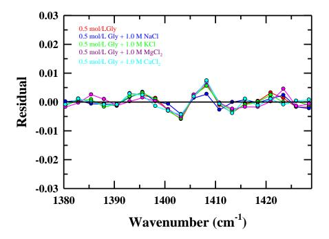
**Fig. S5:** Residuals for the Voigt fit of the experimental Raman spectroscopy data for glycine solutions having 1.0 mol/L salt concentration. Presentation is color-coded.
