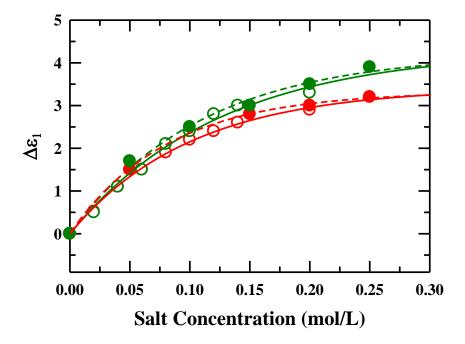
Fig. S4: Salt concentration dependence of  $\Delta \varepsilon_1$  for  $MgCl_2$  and  $CaCl_2$  solutions. Filled circles (red for  $MgCl_2$  and green for  $CaCl_2$ ) represent data for solution containing glycine and open circles represent data for solutions without glycine. Lines (continuous lines for without glycine and dashed lines for with glycine) passing through the data points represents exponential rise to a maximum fit ( $y = a(1 - e^{-bx})$ ).
