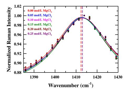
Fig. S6: Experimental and fitted (Voigt) RS data for  $COO^-$  symmetric stretching mode of glycine in glycine (0.5 mol/L) containing  $MgCl_2$  solutions. Presentation is color-coded.
