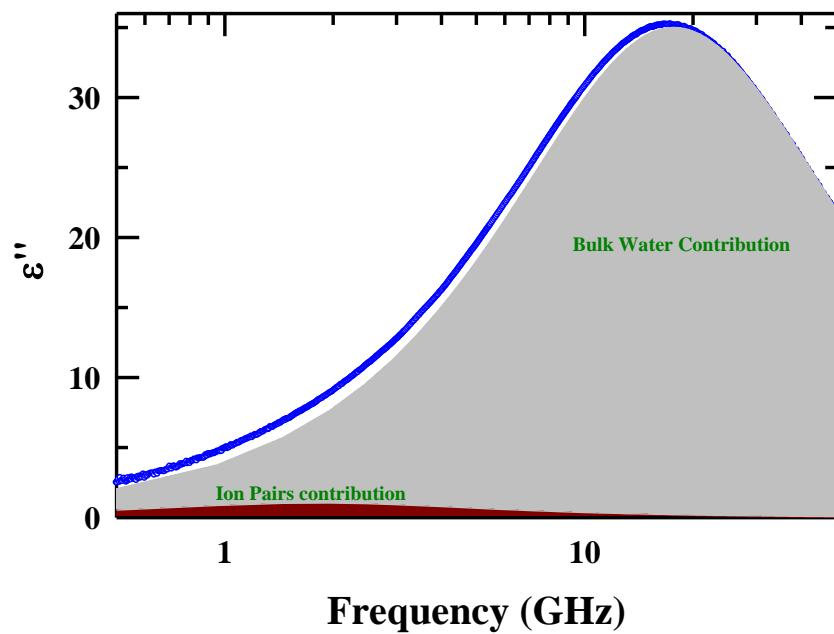
**Fig. S3:** Imaginary part of the complex dielectric response of 0.1 mol/L aqueous  $MgCl_2$  solution. Different DR contributions are represented by color coding.
